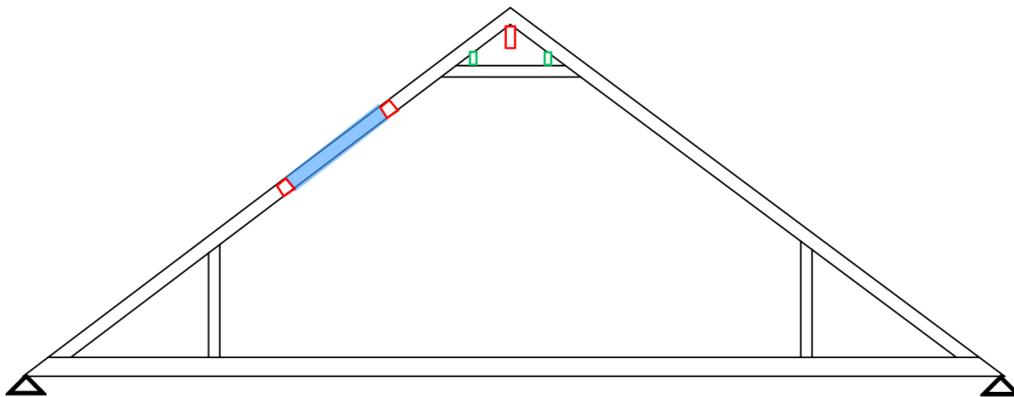
**c) Cut truss supported by velux bridles, ridge beam and purlins at hanging post-rafter connection (i.e. at every node point)**
