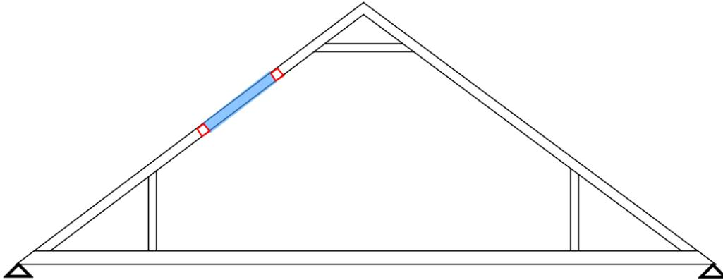
**b) Cut truss supported by velux bridles and ridge beam (or top hat beams)**
