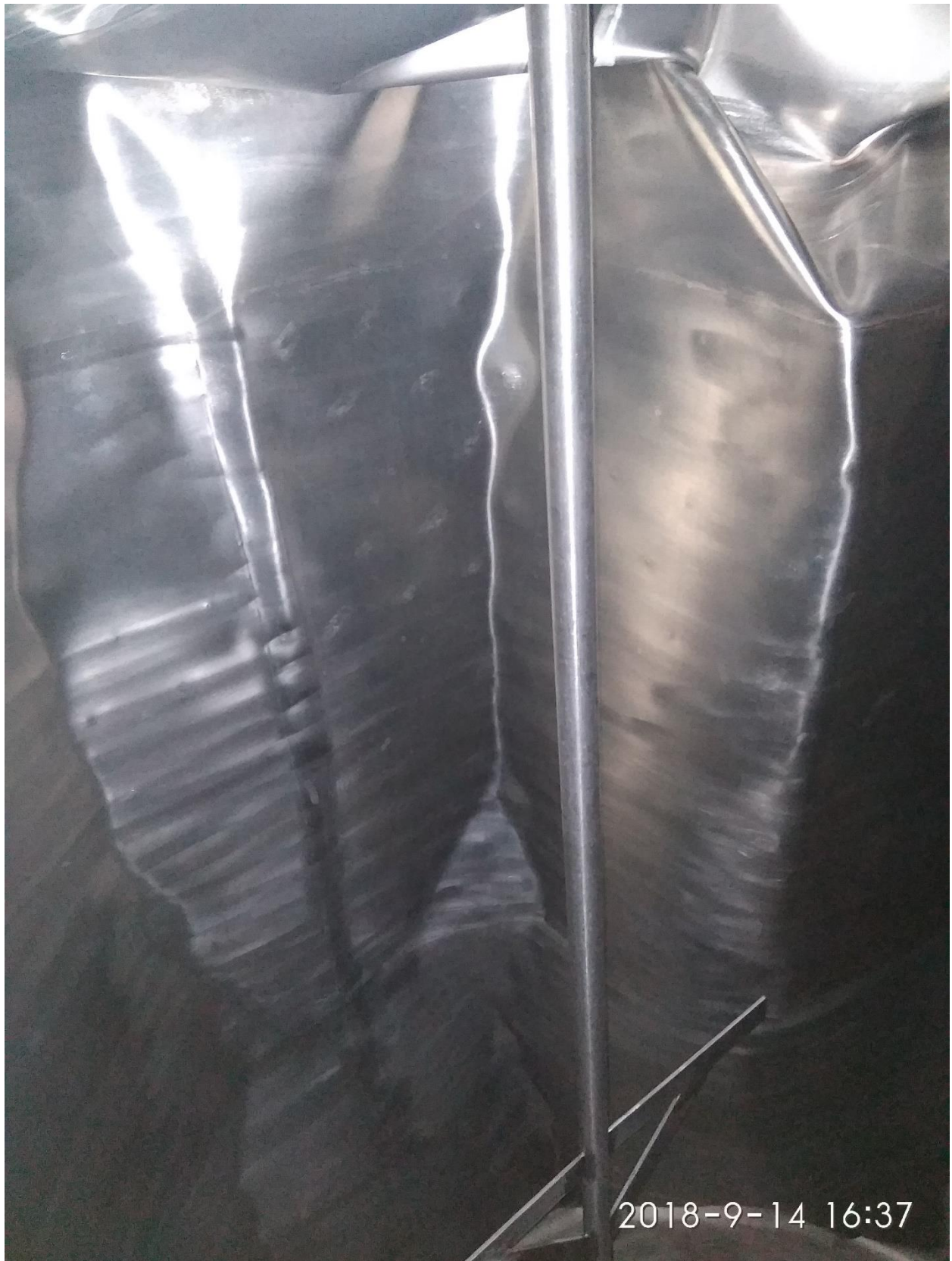
Internal Damage at Chilled water supply & return line nozzles area
