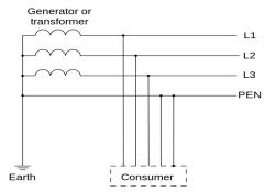
TN-C: combined PE and N conductor all the way from the transformer to the consuming device.
