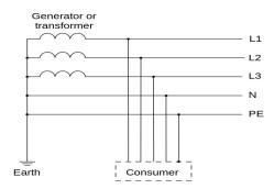
**TN-S**: separate protective earth (PE) and neutral (N) conductors from transformer to consuming device, which are not connected together at any point after the building distribution point.
