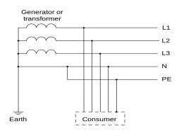
**TN-C-S earthing system**: combined PEN conductor from transformer to building distribution point, but separate PE and N conductors in fixed indoor wiring and flexible power cords.
