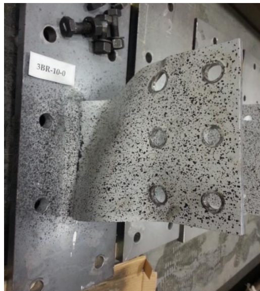
Figure 2-3: Out-of-plane deformation of extended shear tab specimen with stiff support (Salem et al. 2016)
