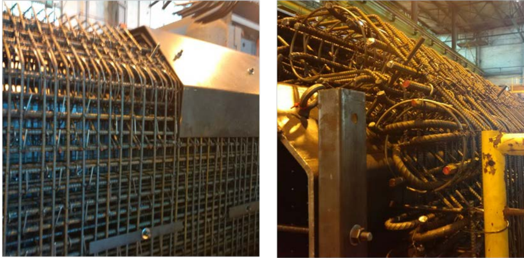
Figure 9.10 Images of Hardened RC Tower Specimen Steel Reinforcing Cage
