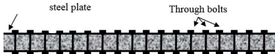
Figure 9.23 Illustrating Recommended RC Tower Panel Retrofit, Section View [128]
