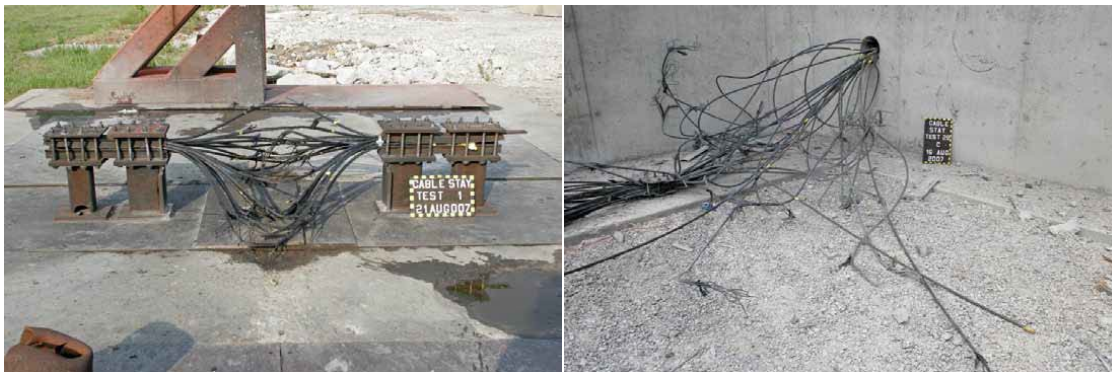
Figure 10.10 Examples of Cable Failure Due to Diamond Charge; Left: Failure of 25% of Strands; Right: Complete Failure of Cable [135]
