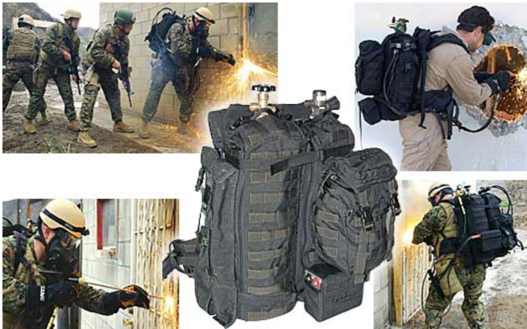
Figure 10.15 Exothermic Torch in Use [145]
