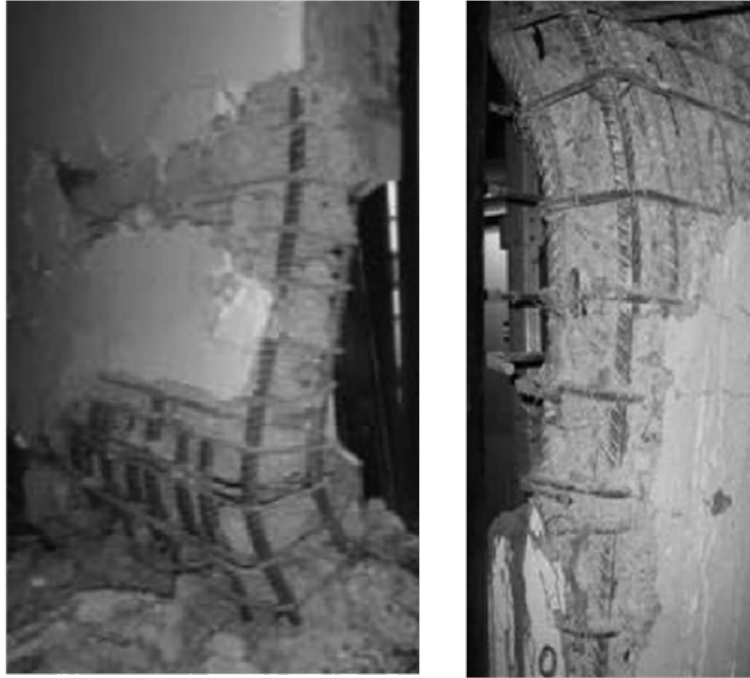
Figure 9.8 Illustrating Component-Level Buckling of Reinforced Concrete Panels Following Extensive Concrete Damage [132]
