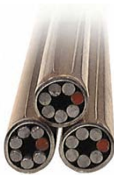
Figure 10.14 Cross Section Exothermic Torch [144]
