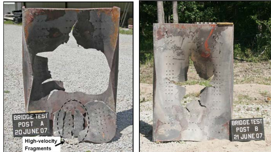
Figure 5.11 Local Breaching Failure of Steel Bridge Tower Test Specimens [93]
