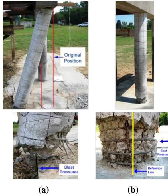
Figure 7.8 Shear-Dominated Behavior of Quarter-Scale RC Bridge Column Specimens Subjected to Standoff Detonations [25]: (a) Direct Shear Failure at Column Base, (b) Dynamic Shear Behavior
