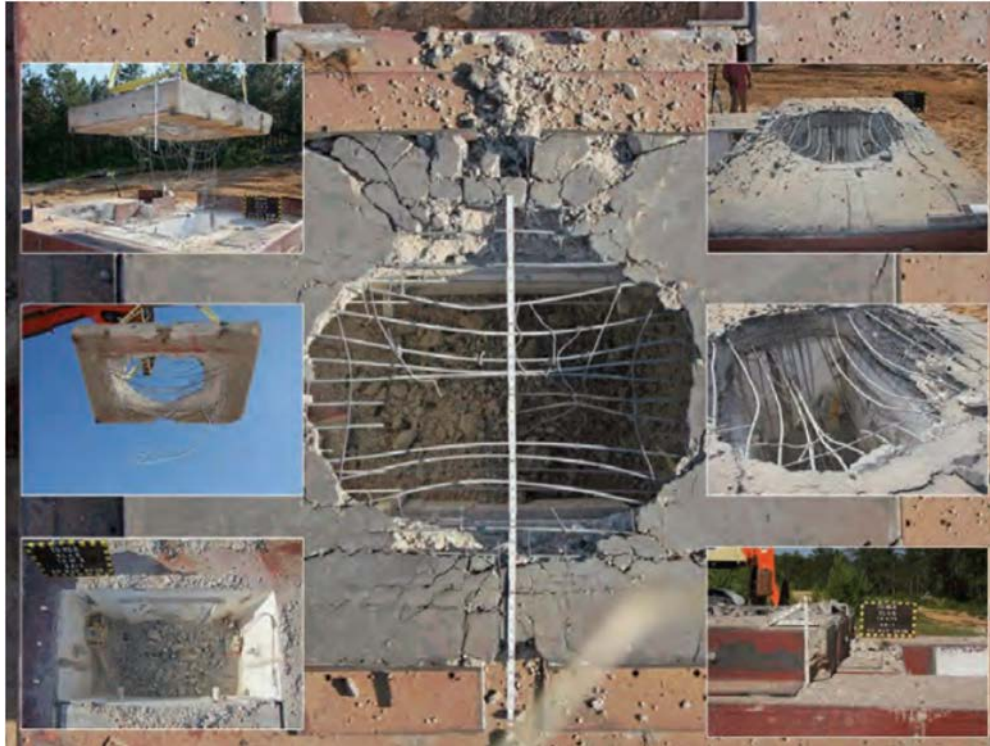
Figure 9.5 Post-Test Images of Close-In Blast Test against Scaled RC Tower Panel Specimen Showing Significant Breach Damage [127]
