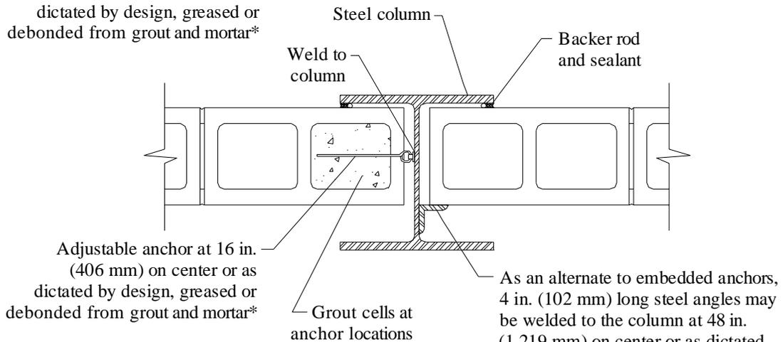
\*The selected anchor should permit in-plane horizontal and vertical movement between the column and masonry while preventing out-of-plane movement perpendicular to the wall surface.
