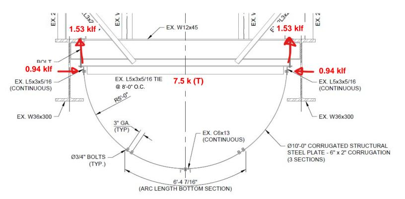
Top connection (flume to continuous angle) - shear rupture:
