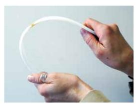
and splits in plastic canoes and kayaks. To test G/flex<sup>®</sup> for this type repair, we simulated splits in the bottom of a thermal formed plastic hull by edge gluing <sup>1</sup>/<sub>8</sub>" thick high-density polyethylene (HDPE) sheets.
