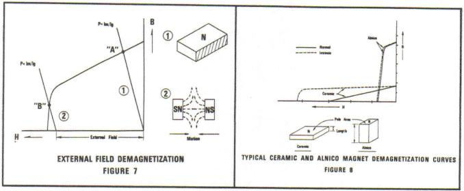
In terms of magnet geometry, high coercive force permits designers to use shorter magnet lengths (distance between poles), whereas high induction permits smaller magnet cross-sections (pole areas). High coercive force also offers greater resistance to external demagnetizing fields.
