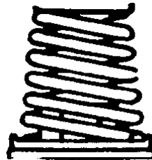
Figure 2-1. Speeder Spring
