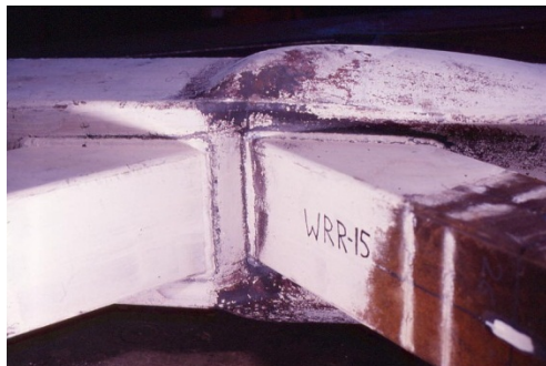
Chord side wall buckling
