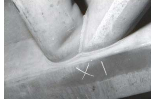
Chord or bracing localised buckling
