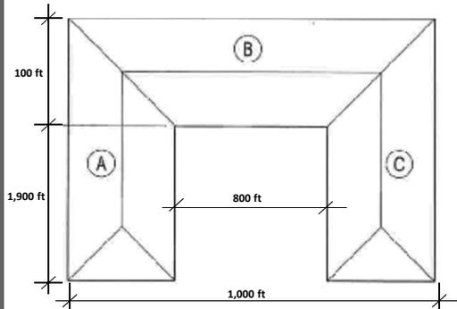
Using full building dimensions for determination of Leeward Wall  $C_p$  is not appropriate in this case
