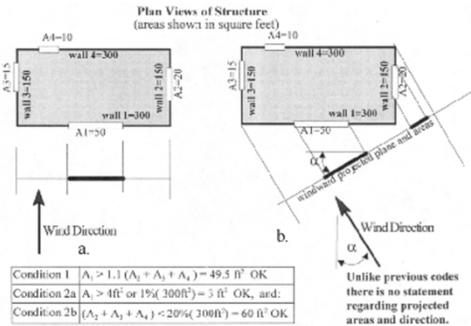
Wind Loads on Non-Standard Building Configurations
