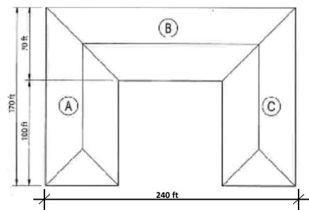
Used full building dimensions for determination of Leeward Wall  $C_p$
