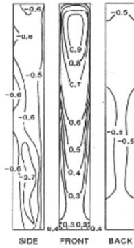
(a) External pressure coefficients measured in wind tunnel.
