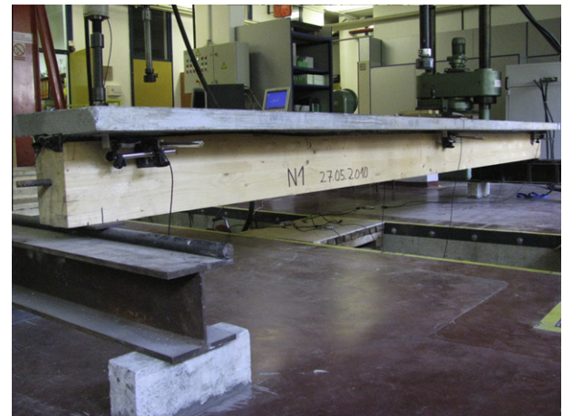
Fig. 7. Installation of the measuring instruments.
