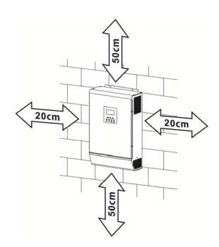
Install the unit by screwing three screws. It's recommended to use M4 or M5 screws.
