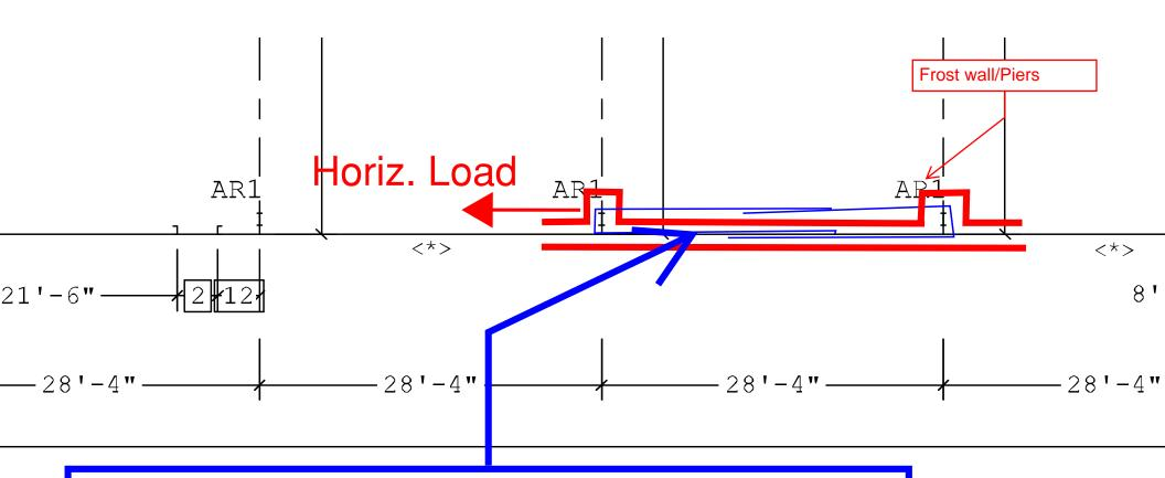
Horiztonal tie rods around anchor bolts in frost wall and poured slab that ties the anchor bolts back to adjacent column and counts on developmental length and dead weight to resist
