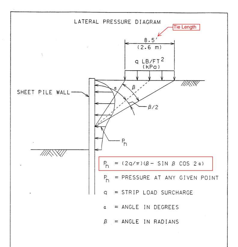
LATERAL PRESSURE DUE TO STRIP LOAD
