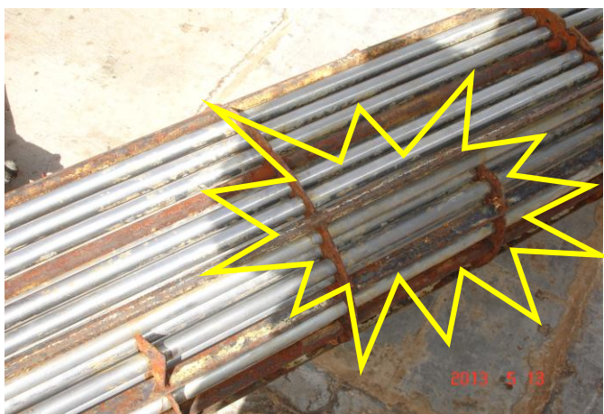
The baffles and tie rods are corroded
