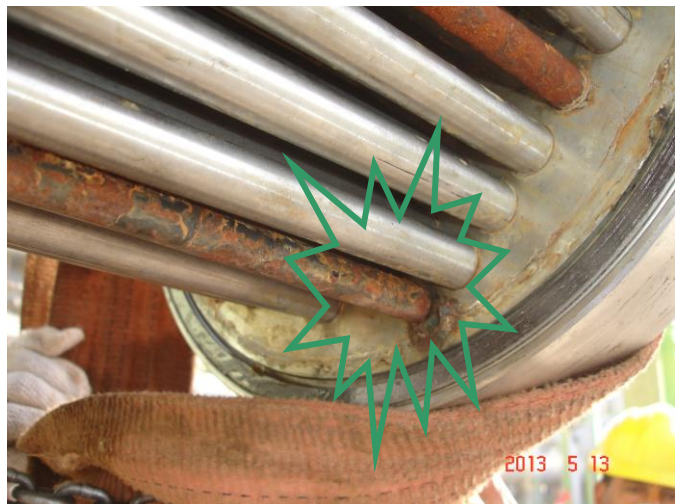
corrosion of a tie rod
