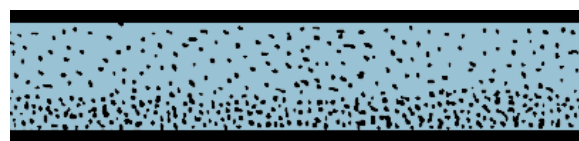
b. Heterogeneous flow. The solids are carried by the fluid, but not distributed evenly.
