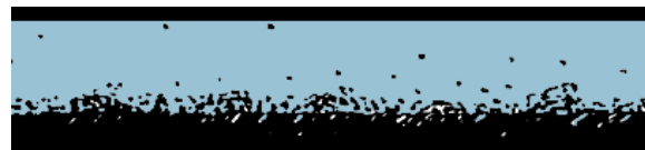
d. Stationary bed flow. Some of the solids do not move.
