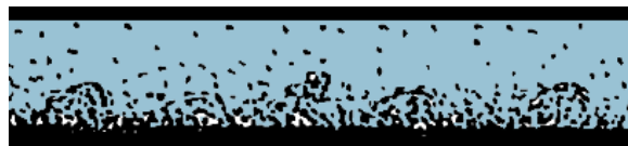
c. Stratified flow. The solids move, but partly along the bottom of the pipe.
