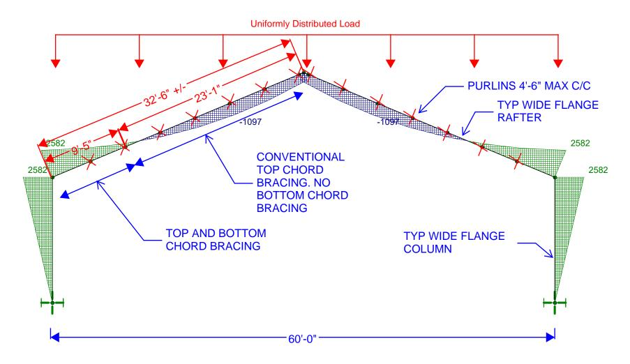
QUESTION: WHAT IS THE UNBRACED LENGTH OF THE COMPRESSION FLANGE OF RAFTER AT COLUMN WITH NEGATIVE MOMENT? 4'-6"? 23'-1"?
