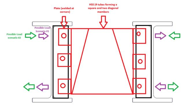
RED FRAME WORK IS WELDED AND CONNECTED TO STIFFNER VIA BOLTS
