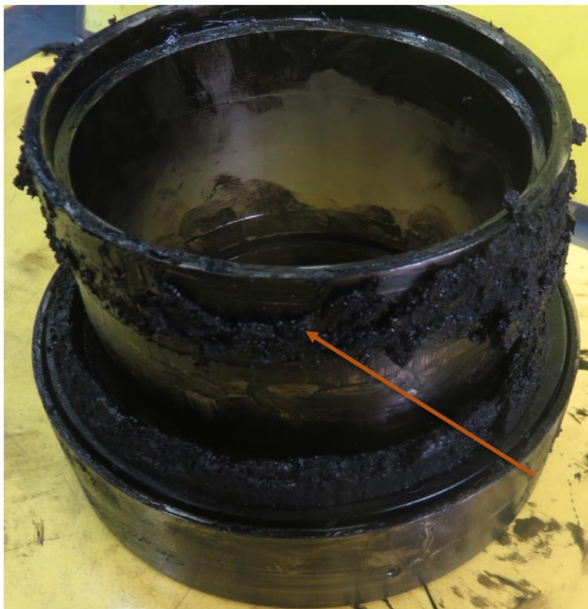
Sleeve (Pos # 12) OD under the outboard bellows area is covered with thick layer of sludge deposits.
