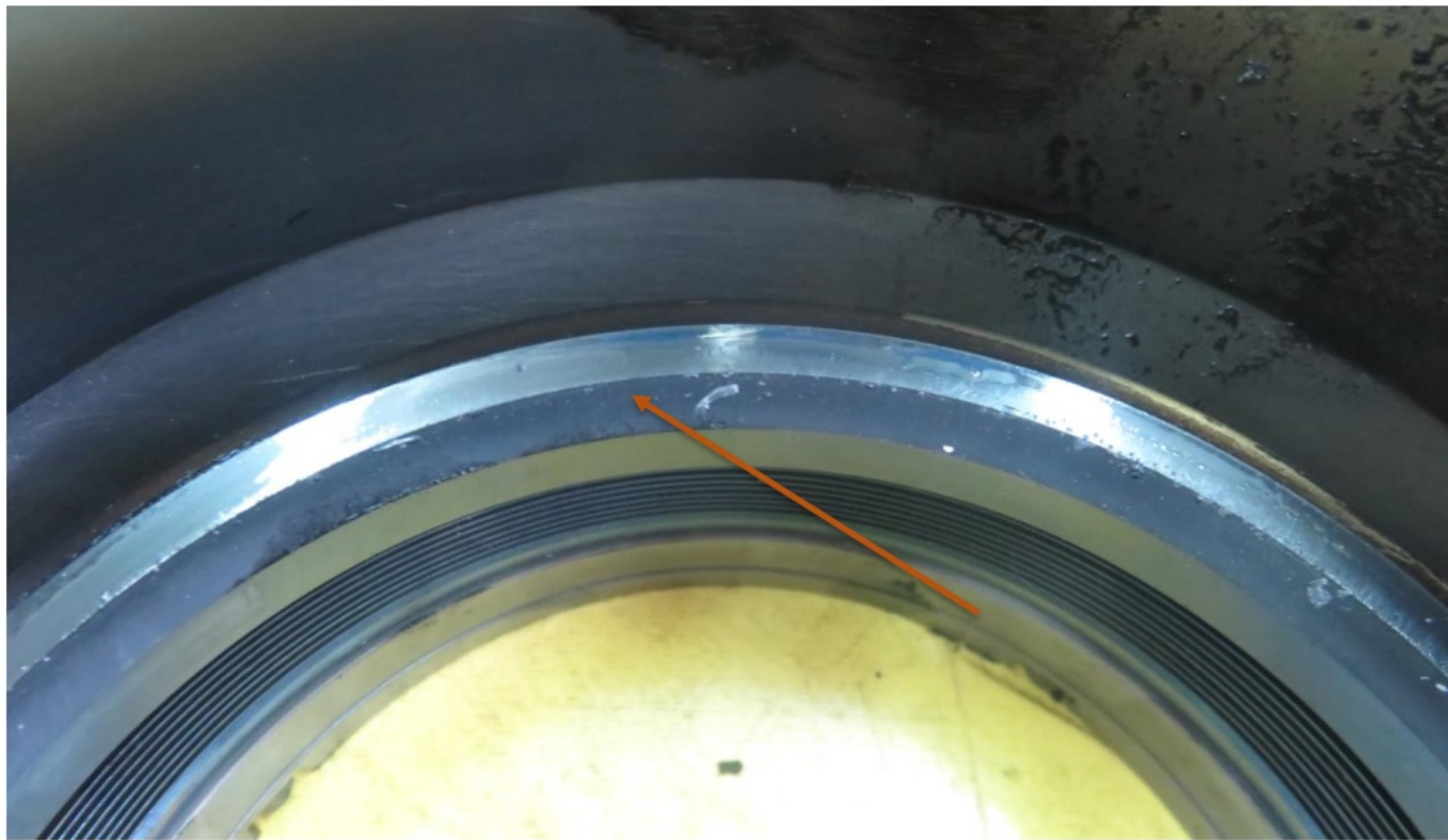
Inboard bellows (Pos # 1) shows hard debris.
