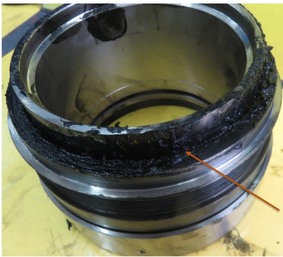
Outboard bellows (Pos # 6) observed stuck on the sleeve OD.
