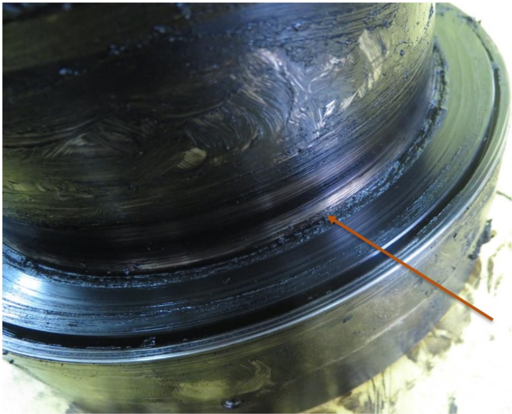
OB Mating ring (Pos # 8) ID area is full of hard coke deposits.
