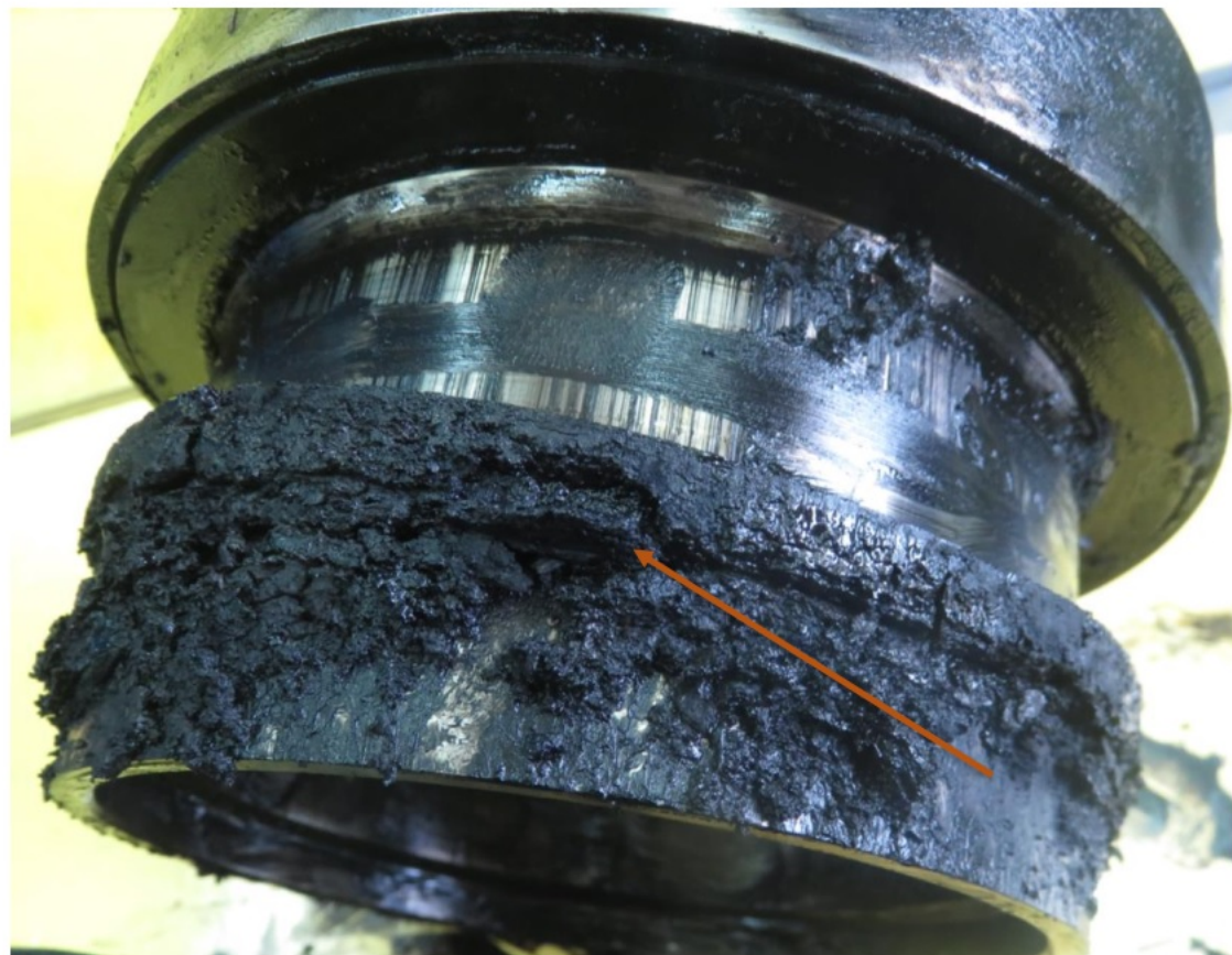
Sleeve (Pos # 12) OD under the outboard bellows area is covered with thick layer of sludge deposits.
