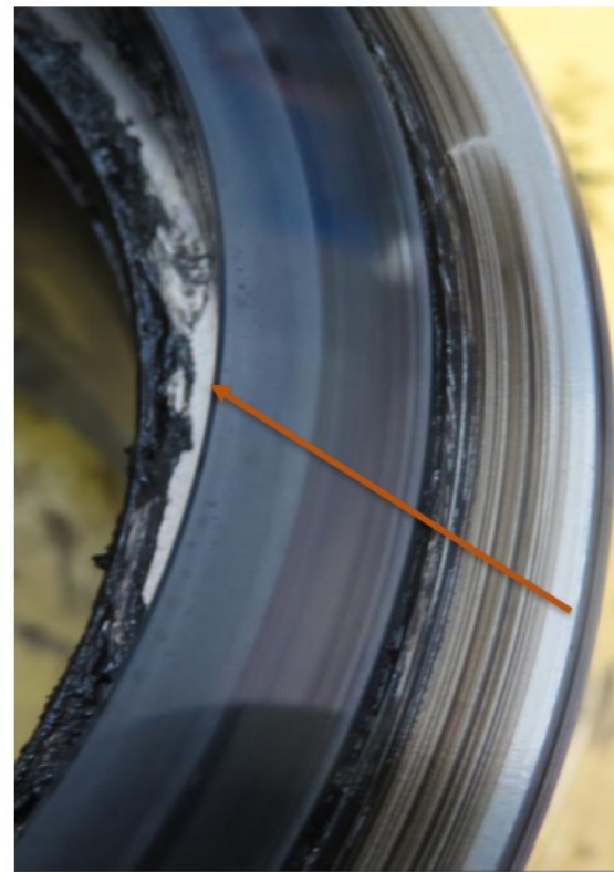
IB Mating ring (Pos # 4) shows gramophonic wear marks.
