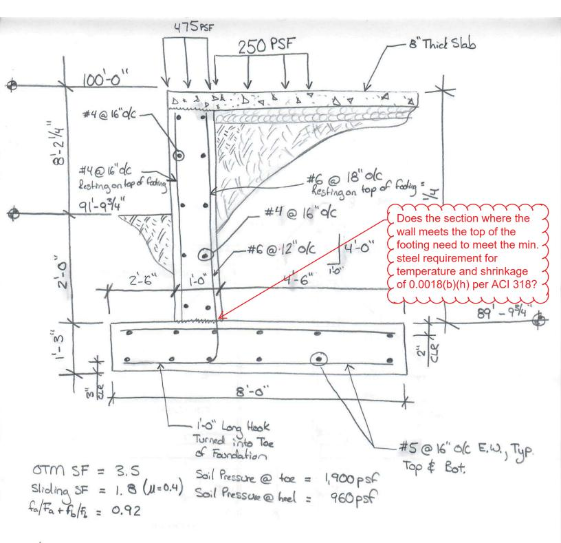
fc = 3,000 psi Soil Bearing Pressure (Allowable) = 2,000
