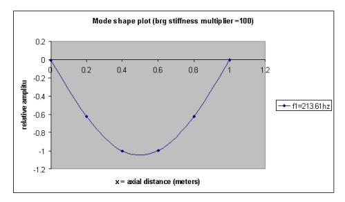
We can check the frequency for this mode (first mode at multiplier =100) using a simply-supported beam calculation, which gives a frequency of 214.21 hz. This is reasonably close to the program-calculated resonant frequency of 213.6hz.
