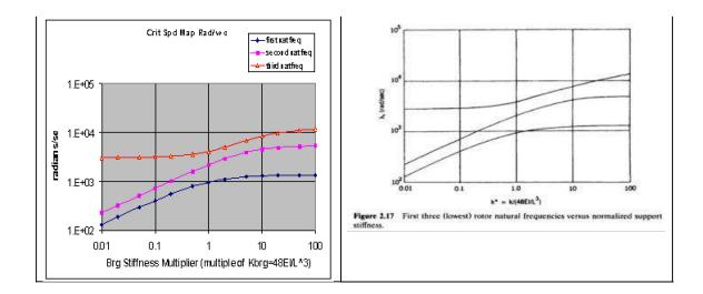
Looking toward the left of the critical speed map, we suspect that the first two modes increasing linearly on log-log plot with a slope of 0.5 are rigid-rotor modes. We confirm this with a modeshape plot of these first two frequencies (bearing multiplier 0.01):
