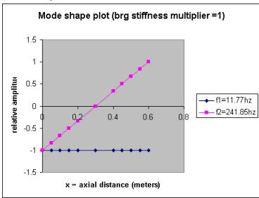
Pilkey's wc1 corresponds to the first mode f1 at 11.77hz where the rigid rotor moves parallel to it's axis with a very simple solution w=sqrt(Ktotal./M).
