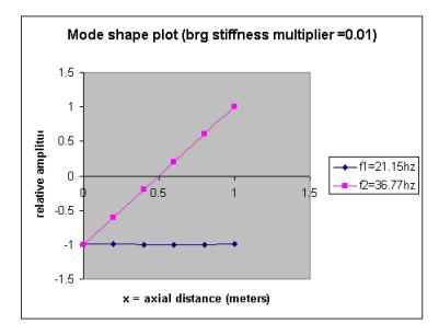
With the rigid rotor simplification, we can analytically verify the first two resonant frequencies at a bearing stiffness multiplier of 0.01.
