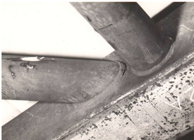
Figure 1: Round branch-to-rectangular/square chord welded connections
