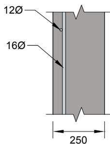
$d = 250 - (30 + 12 + 8) = 200$  mm. At the plate perimeter, the effective depth is taken to the back of the plate ie  $d = (200 - 30) = 170$  mm. It is conservative to use this value for the basic control perimeter  $u_1$ .
