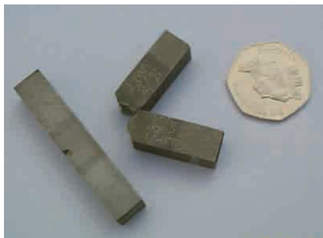
Below: Charpy V-notch impact test piece
