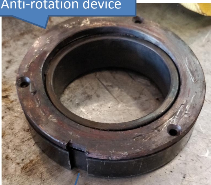
Grease path to roller bearing restricted by locking bolt
