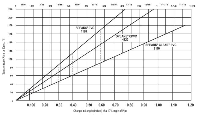
Highly important is the change in length of plastic pipe with temperature variation. This fact should always be considered when installing pipe lines and allowances made accordingly.
