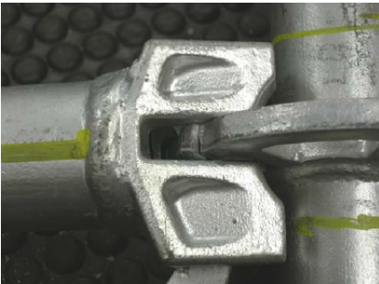
FAILURE OF ROSETTE AT 11,811 LBS.
