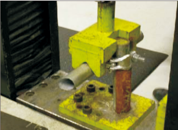
RIGHT ANGLE COUPLER TEST CONFIGURATION
