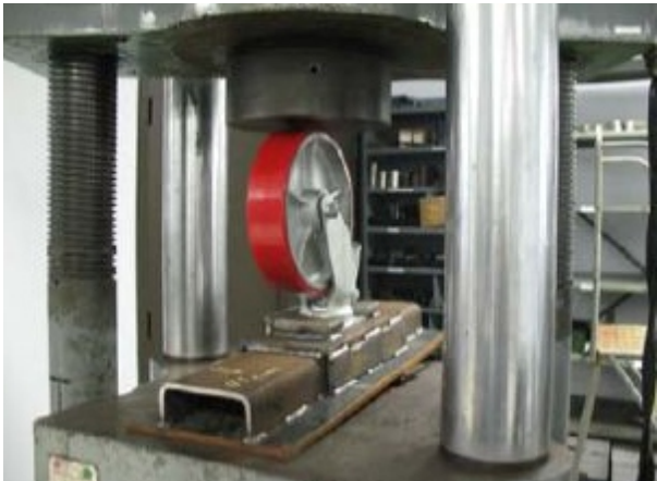
LOAD APPLICATION AT 5°AXIAL OFFSET
