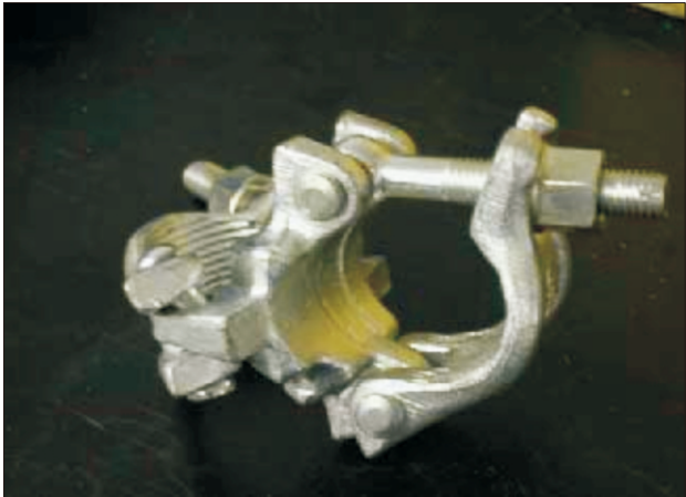
RIGHT ANGLE # 1 . ULTIMATE LOAD OF 14,580 LBS.
