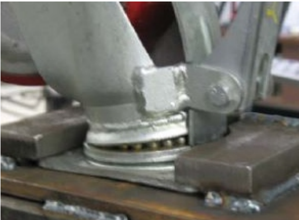
TYPICAL STEM DEFLECTION FAILURE FOR EACH CASTER
