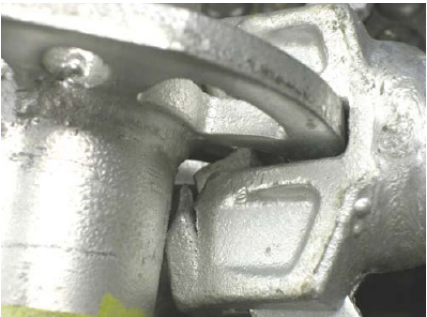
FAILURE OF WEDGE AT 14,173 LBS.
