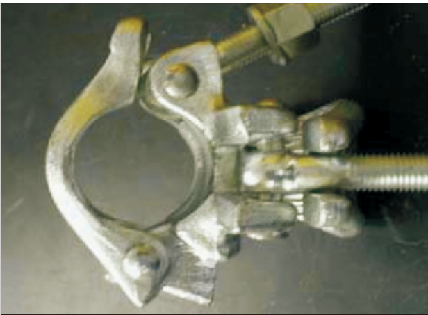
RIGHT ANGLE # 2, ULTIMATE LOAD OF 15,150 LBS.
