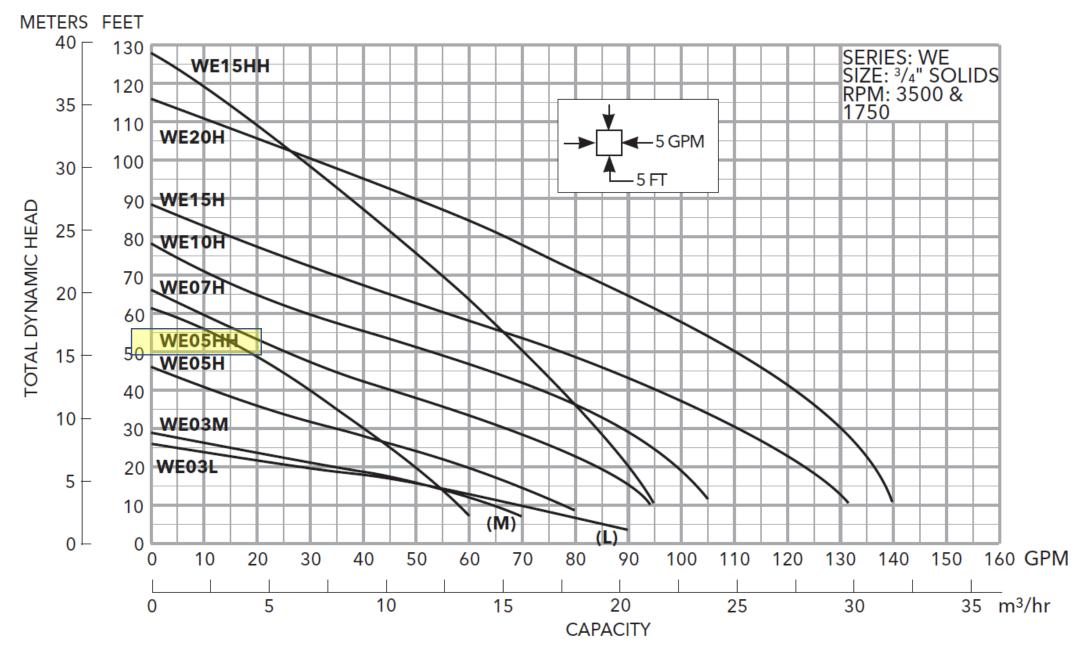
Calculate fluid power from previous pump curve (FHP = gpm\*hd/3960). Peaks at 0.31hp. With 0.54 pump efficiency this would create a BHP demand of 0.57bhp on the output of the motor which exceeds the steady state rating 0.5hp. For operation in the middle of the
