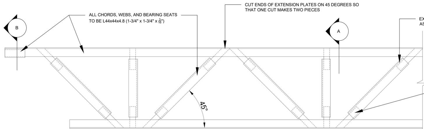
IF DEMANDS DICTATE EXTENSION PLATE CAN BE MADE WIDER ON UNENCUMBERED SIDE OF ANGLE
