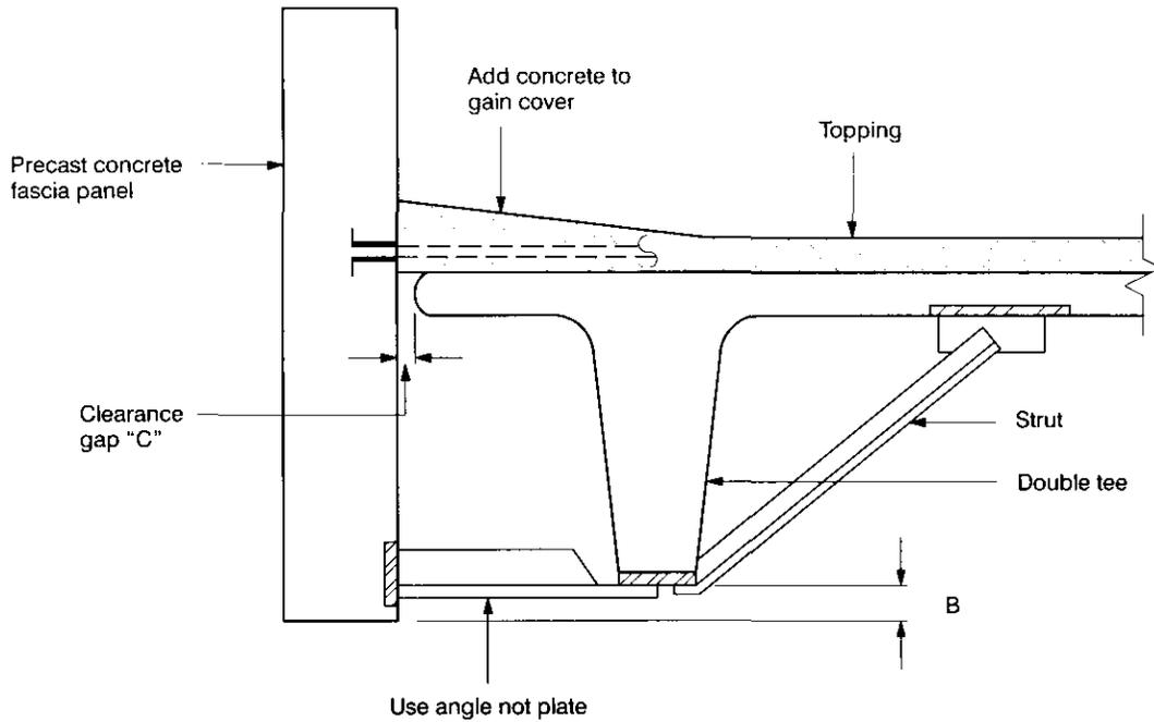
1. Consider locally thickening concrete topping adjacent to fascia panel to accommodate insert placement tolerances and assure concrete cover over bars threaded into insert in fascia panel. This detail can also be beneficial to drainage in this area.
