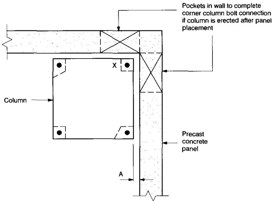
1. Provide pockets in the walls at either of the locations as shown above. Pockets should be sized and oriented to allow execution of bolted connections marked "X". Alternatively provide adequate clearance "A" to provide wrench access necessary to complete the connection at "X".
