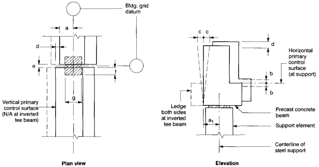
**Precast element to: precast element, cast-in-place concrete, masonry, or structural steel**
