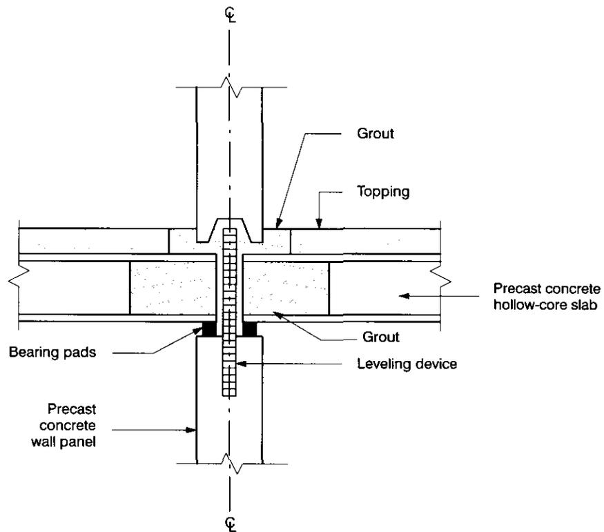
1. Require tighter tolerances than standard for the slab length due to the very small bearing width usually available in the panel framing system for such structures.
