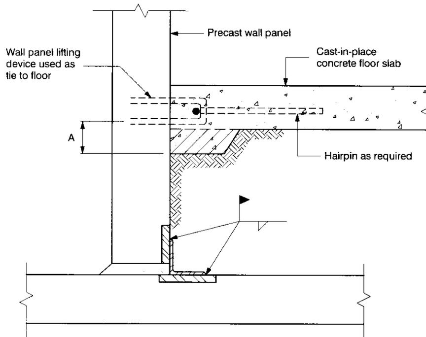
1. When panel lifting device embeddings are used as a tie to the floor, use a placement tolerance of  $\pm \frac{1}{2}$  in. [ $\pm 13$  mm] rather than the larger standard PCI tolerance given for embedded lifting devices when they are only used for lifting.
