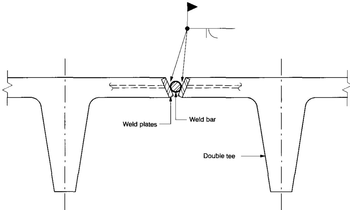
1. Provide flange connection weld plates at an angle as shown above to accommodate tolerances required for plate placement and allow the placement of a proper flare weld. Plate tipping tolerances are less critical for flange connector plates angled as shown compared to the more stringent tipping tolerances required for proper welding connector weld plates oriented with their surfaces parallel to the vertical centerline of the flange to flange joint (see Fig. 18.17.1, Detail B).
