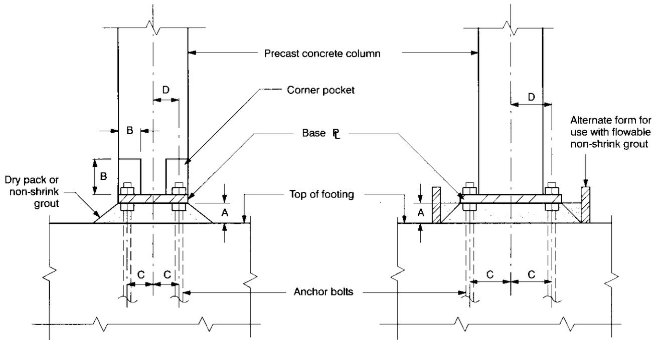
1. Provide clearance "A" to accommodate tolerances required as result of the combination of column length and footing elevation tolerances. This dimension is typically set to accommodate bottom leveling nuts and for proper tamping of dry pack grout.
