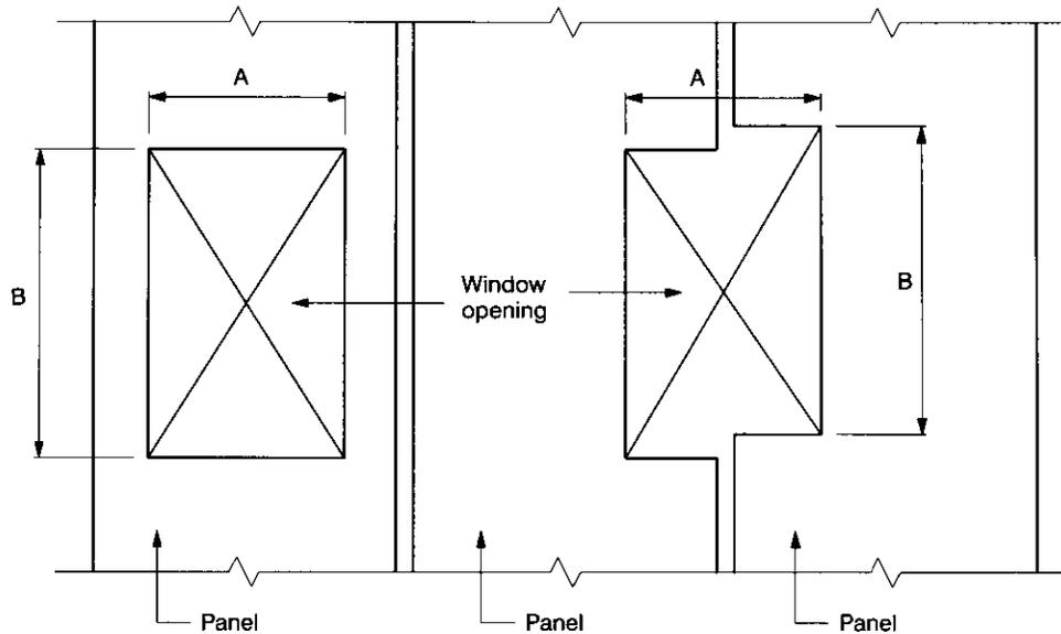
1. Consider the tolerance variations in window width and the minimum required caulking width between the window jambs and the wall panel to determine blockout dimension "A" and the tolerance on the "A" dimension.
