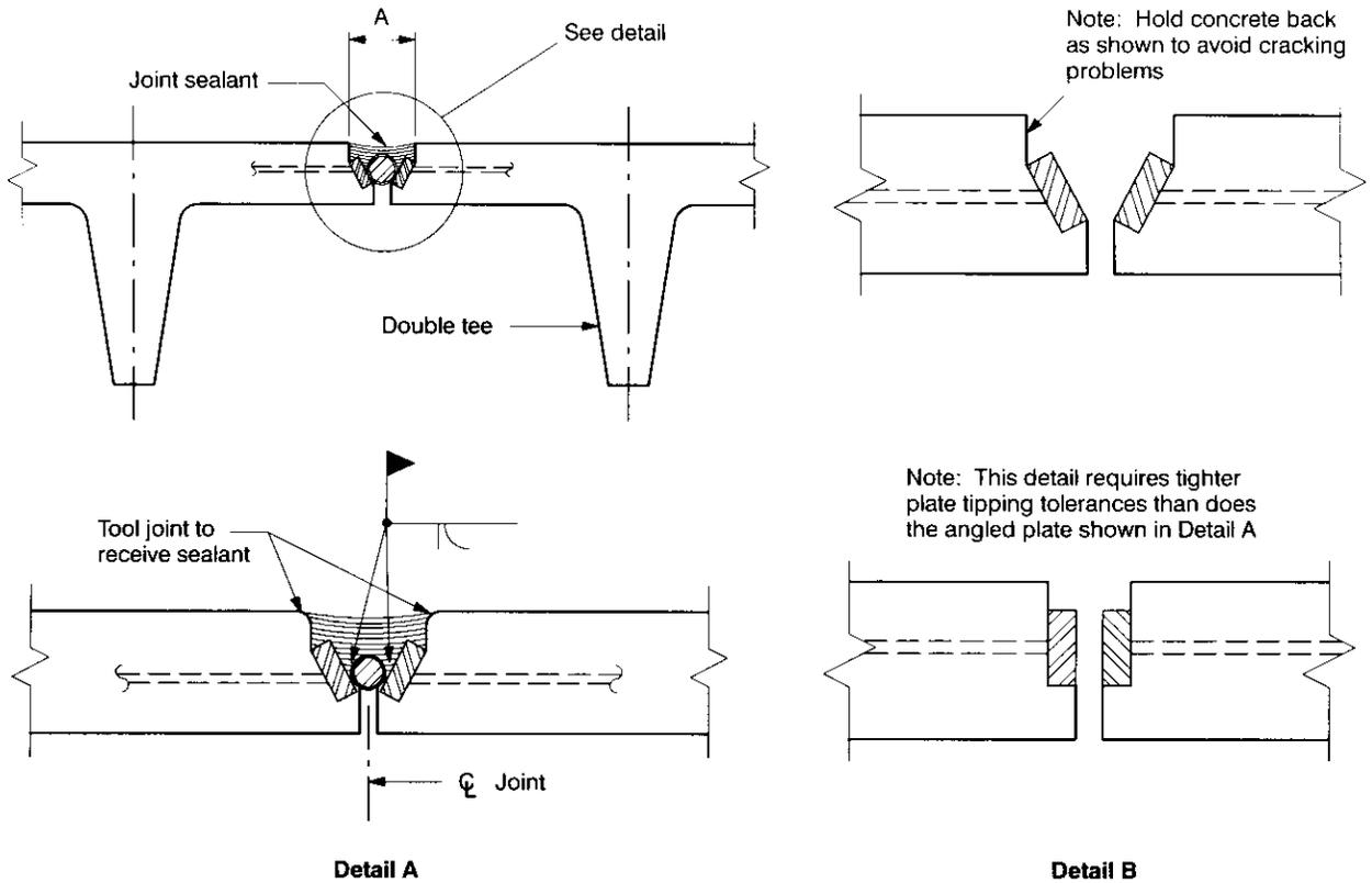
1. Tool edges of tee flange at weld plate locations as shown to assure that there is not a thin section of concrete directly above the weld plate that will be prone to cracking because of thermal expansion of the plate during welding. This can result in failure of the sealant system.
