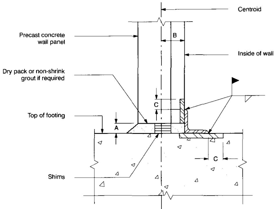
1. Provide clearance "A" to accommodate tolerances as result of the combination of panel length and footing elevation tolerances.
