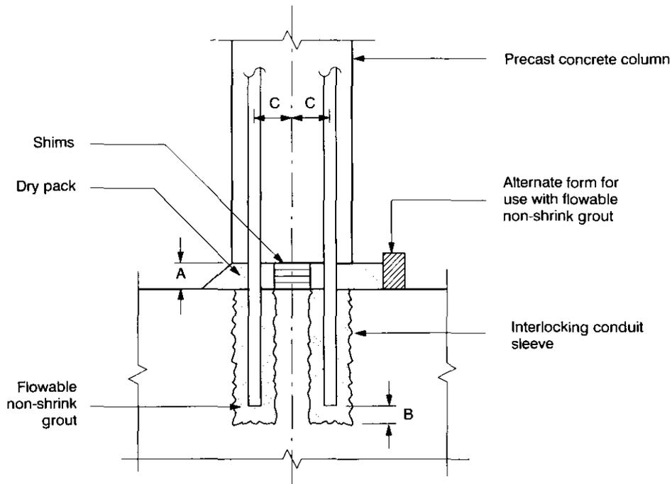
1. Provide clearance "A" large enough to accommodate tolerances required as result of the combination of column length and footing elevation tolerances.
