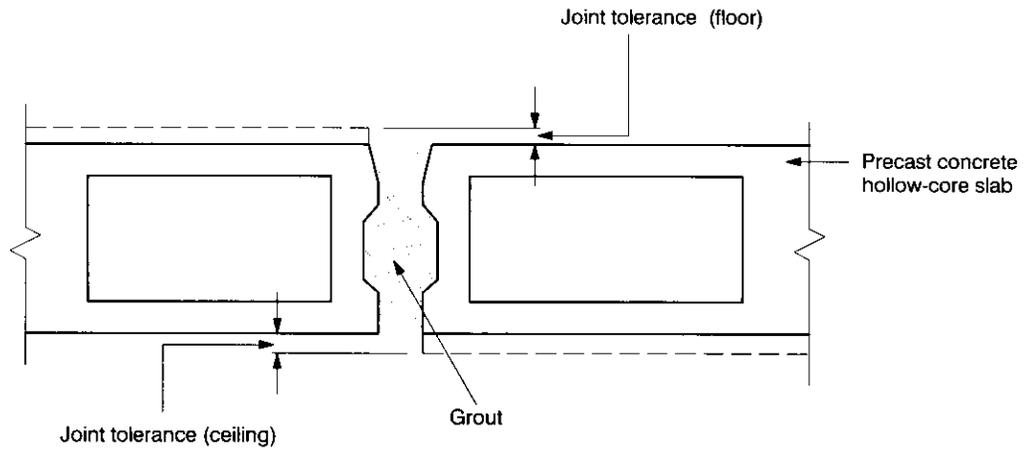
1. Use leveling devices to level the bottom edges of hollow core slabs at the joint location to minimize the effects of any differential camber when the ceiling is to be exposed or planned to receive direct acoustical treatment on the ceiling.
