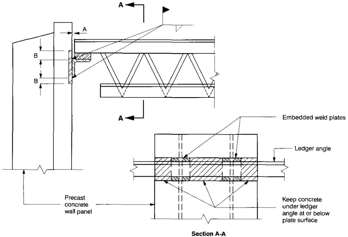
1. Provide adequate weld plates of sufficient size as needed to accommodate the combined effects of erection tolerances for the wall panel and embedded weld plate location and still provide adequate plate projection "B" to allow proper welding.
