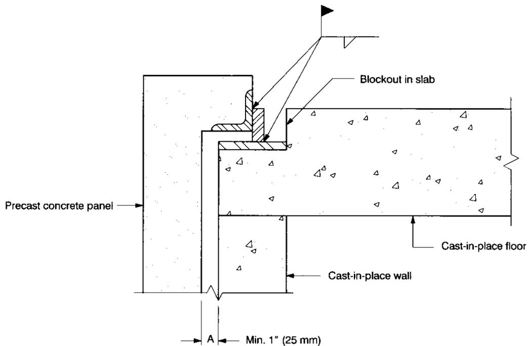
1. Provide a minimum of 1 in. [25 mm] clearance "A" to accommodate the tolerances from a combination of the panel thickness and the edge location of the cast-in-place slab and wall. If the minimum 1 in. [25 mm] clearance is used, care must be taken with dimensioning and detailing to assure that the cast-in-place and precast tolerances allow proper fit up without the requirement for rework.
