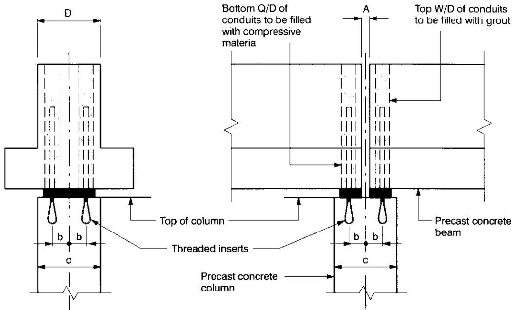
1. Use embedded conduits with oversized diameter to accommodate tolerances required for insert placement in the column.
