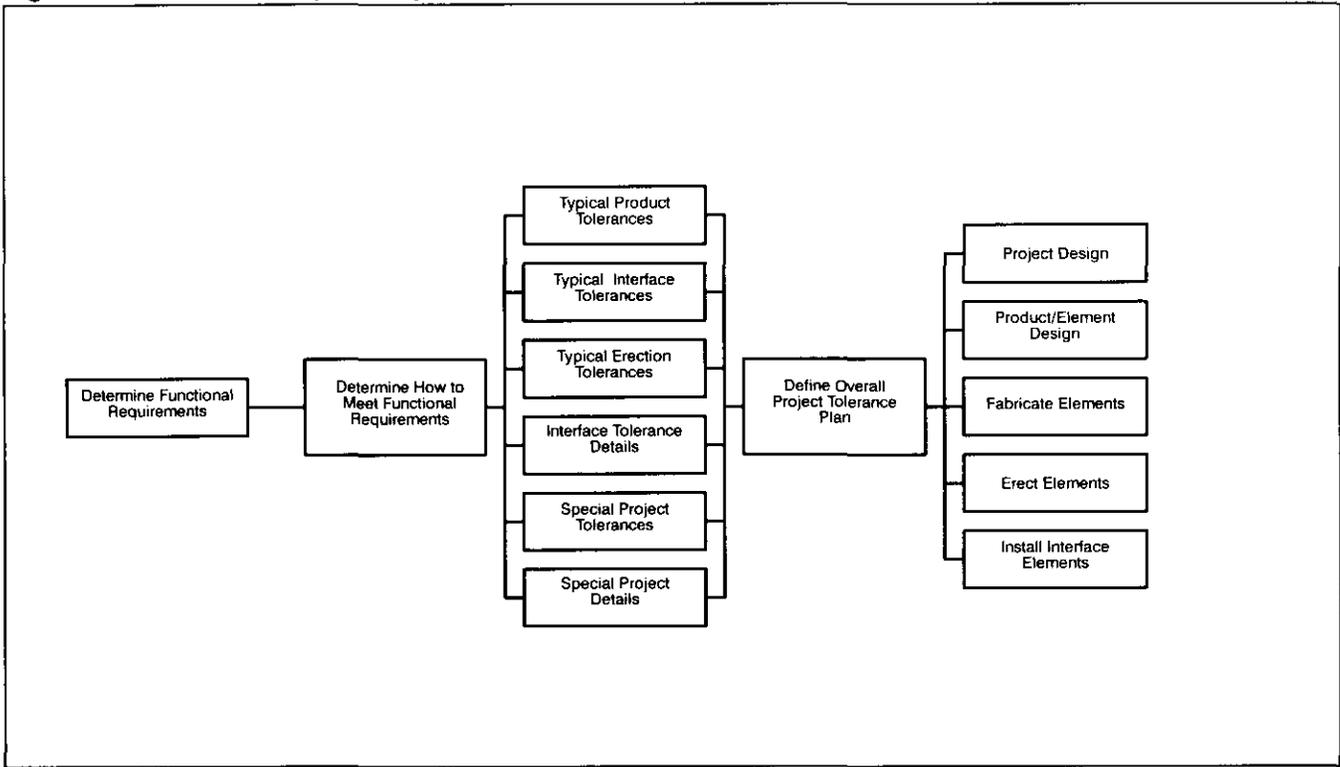
**Fig. 1.4.2 Specifying Tolerances—Precaster Design-Build Contract**
