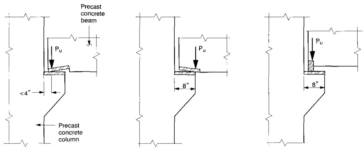
Beam bearing tipped; minimum haunch eccentricity
