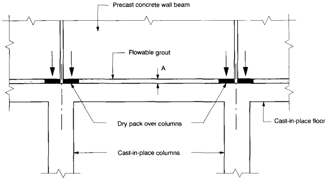
1. Provide adequate clearance "A" to accommodate cast-in-place concrete floor tolerance and assure that panel loads are transferred at column points only as shown above. This is necessary to avoid unintended loading of the floor slab and eccentric loading of the supporting columns.
