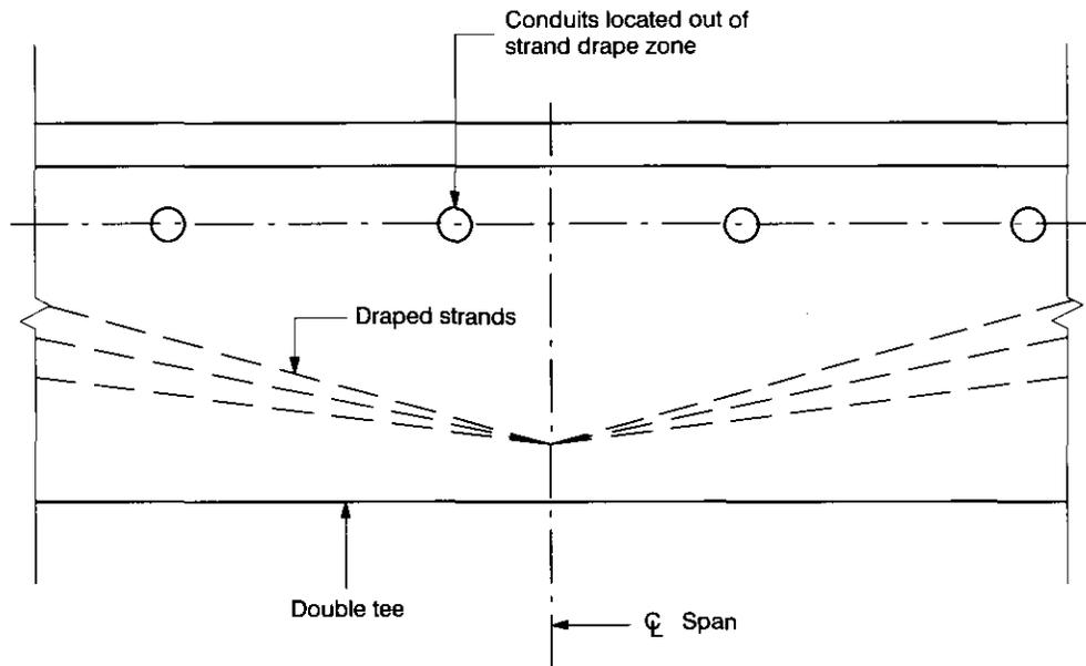
1. Locate embedded conduits above the level of the top strands or establish special project tolerances for lower conduit placement to accommodate the interface of the conduit with the draped strands.
