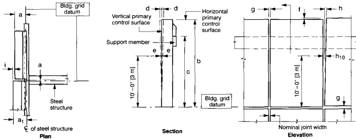
**Precast element to structural steel**
