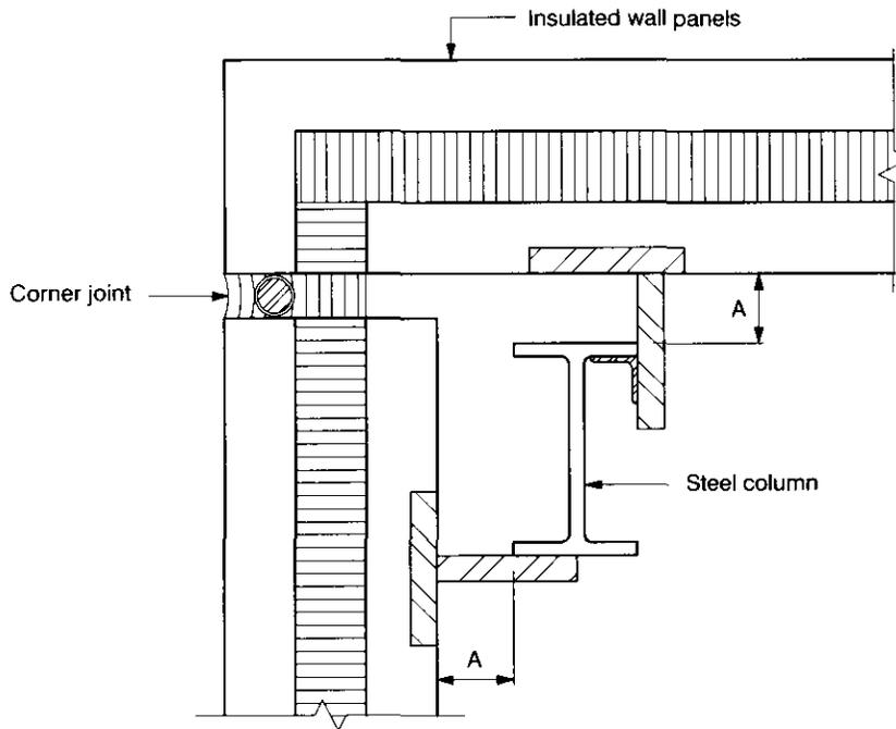
1. Consider the potential for opening of the corner joint as result of thermal bowing of these adjacent panels in different directions. Assure that any calculated joint opening does not exceed the motion capabilities of the specified joint sealant and joint sealant detail.
