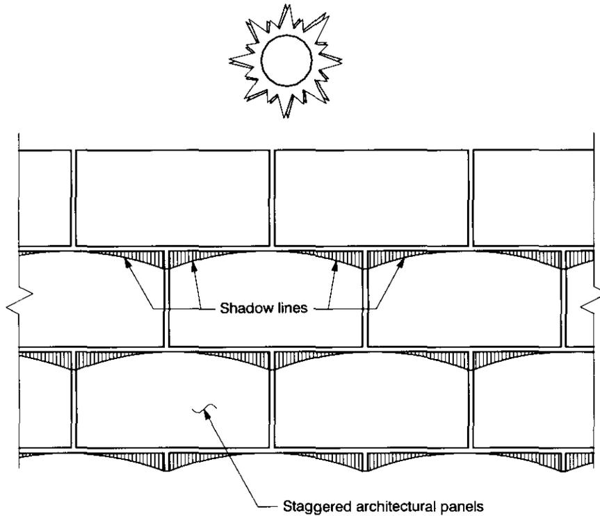
1. Check design of panels to assure that excessive thermal bowing will not be a problem. As shown in the drawing bowing of staggered panels can result in unwanted shadow lines at certain times of the day.
