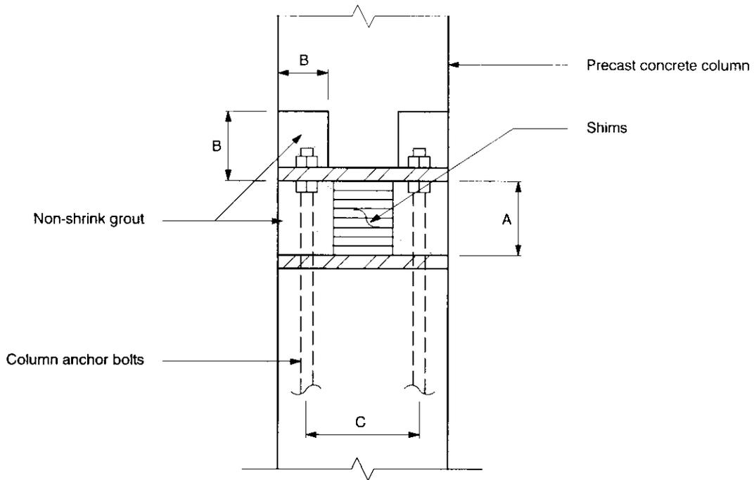
1. Provide adequate clearance "A" to accommodate the tolerances required for column length.
