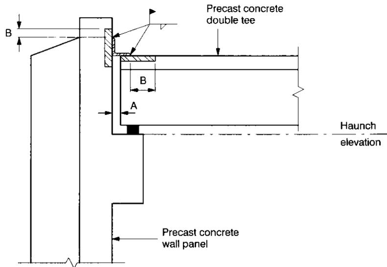
1. To create a visually pleasing line at the top of the panel and ease the erection of the roof elements, the haunch elevation of precast concrete wall panel should be set as a primary control surface. Tolerances for wall length and footing elevation should be absorbed at the panel bottom connection by varying the grout pad thickness.
