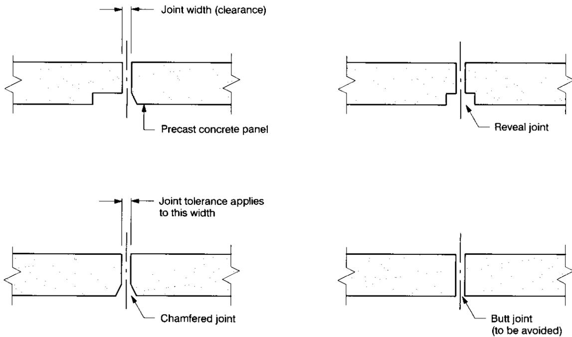
1. Specify either a chamfered or reveal joint, since these types of joints can accommodate the tolerance required for panel thickness and the shadows formed within these joints will minimize any adverse effects on the aesthetic appearance of the joint system.
