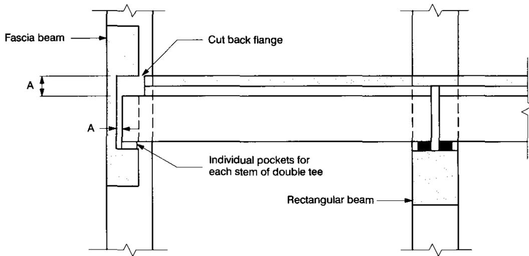
1. Allow adequate clearance "A" at the fascia end of the double tee to assure that the tee stems can be easily slid into the pockets provided in the fascia beam.
