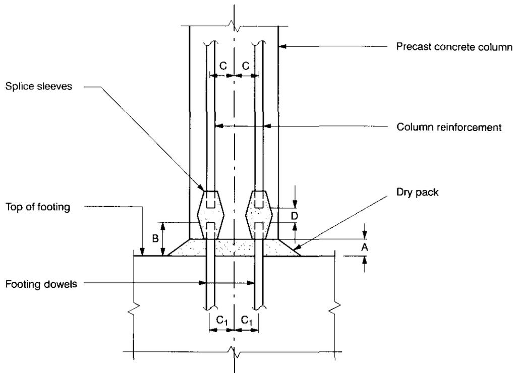
1. Use matching templates for the location of column reinforcement and splice sleeve placement within the footing to control critical dimensions "C" and "C<sub>1</sub>" which should be identical.
