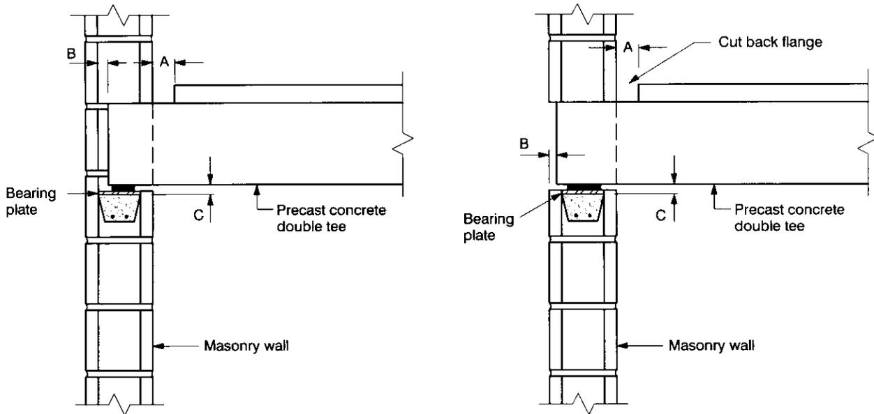
1. Provide adequate clearance "A" to accommodate tolerances required for the vertical alignment of masonry and tee length tolerance. Dimension "A" should be based on ease of erection, forming, and fire resistance considerations.
