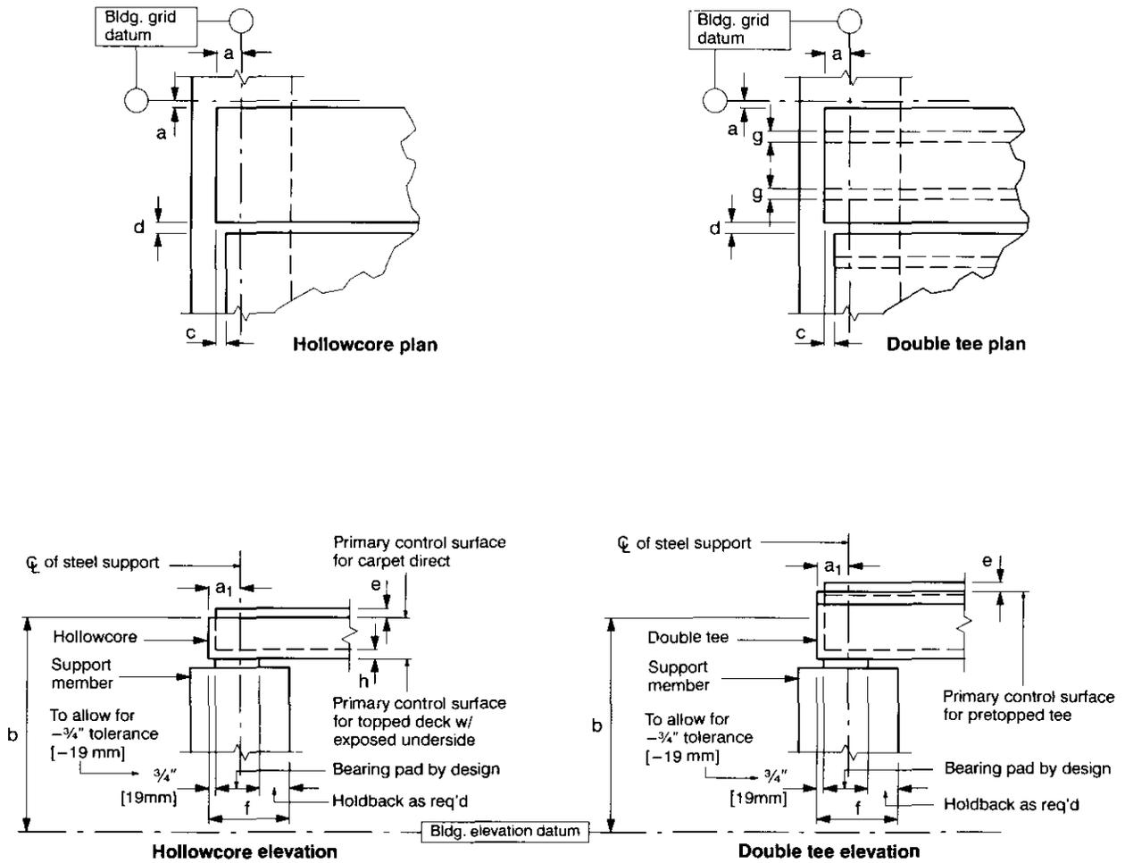
**Precast element to: precast, cast-in-place concrete, masonry or structural steel support**
