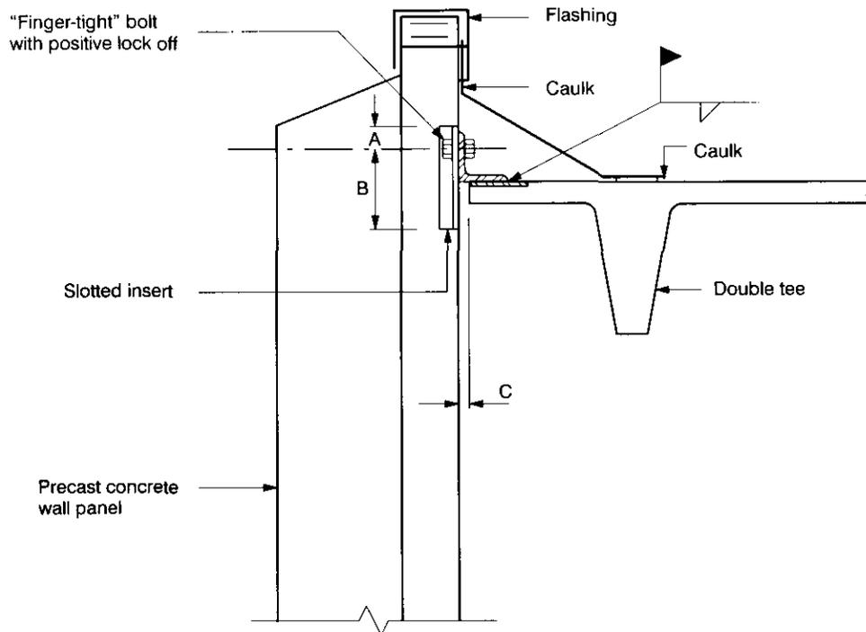
1. Provide adequate insert slot clearance "A" to accommodate anticipated camber growth of tee, including the effects of camber tolerances.
