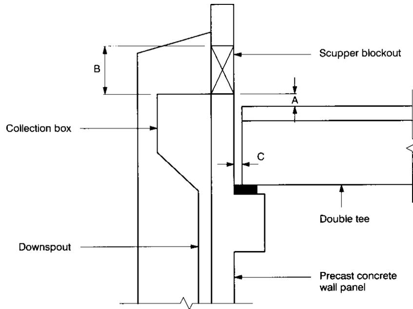
1. Provide clearance "A" to accommodate tolerances resulting from a combination of tee depth, insulation thickness, and roofing material thickness tolerances. When locating scuppers in wall panels oriented parallel to direction of beam span, consider the effects of beam deflection when determining scupper elevation.
