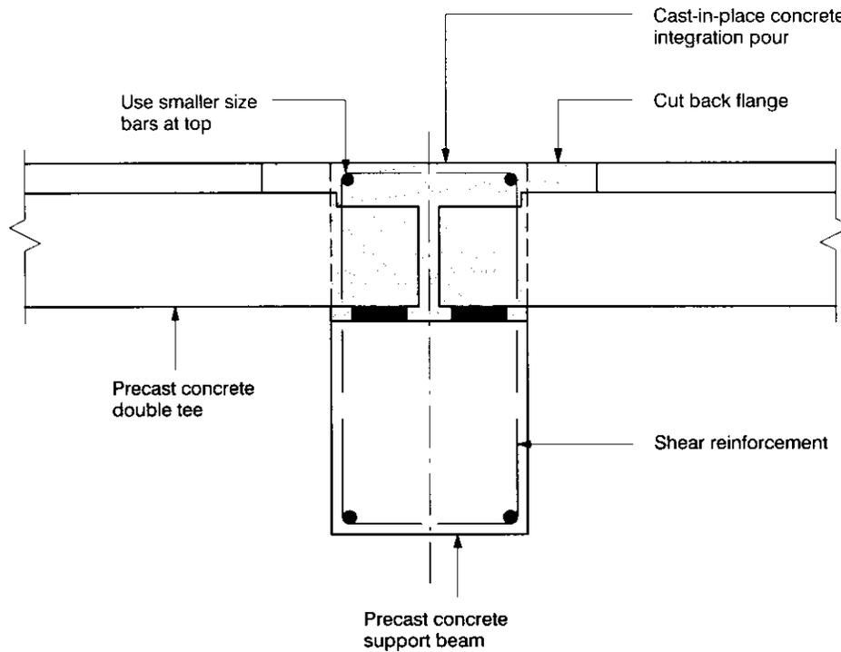
1. In order to avoid conflict between embedded shear reinforcement protruding from the support beam and tee stems, consider the layout of the double tee stems when determining the spacing of the beam shear reinforcement.
