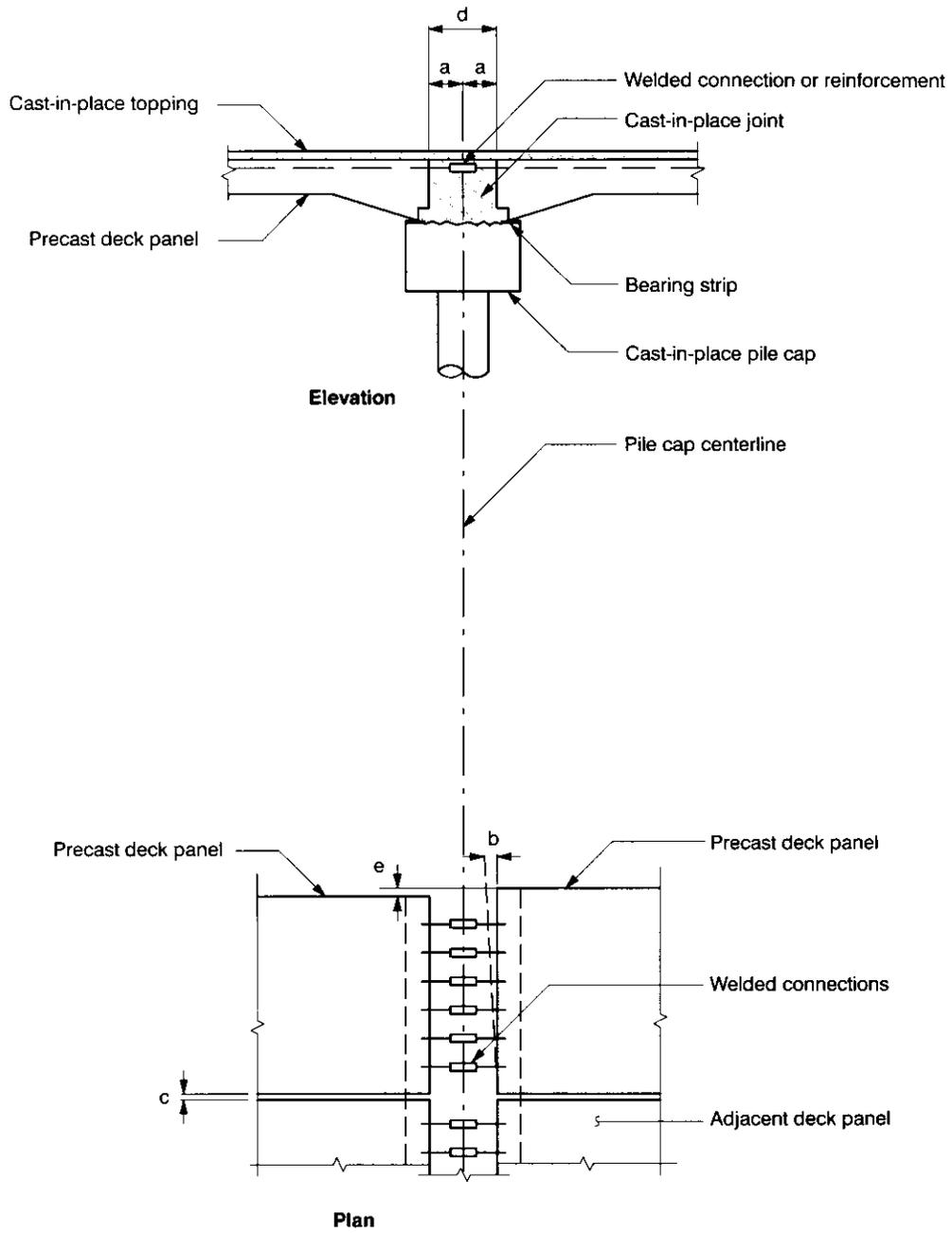
**12.11 Pier Deck Erection Tolerances**
