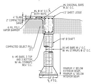
16/48 DRILLED SHAFT; EXTERIOR BEAM W/ STONE LEDGE (NOT TO SCALE)
