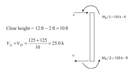
Checking columns B and C for strong column-weak beam considerations.
