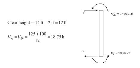
Checking columns B and C for strong column-weak beam considerations.
