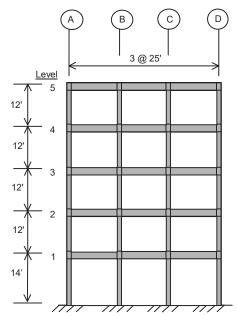
Determine if a Type 5 vertical irregularity—discontinuity in capacity-weak story—condition exists in the first story:
