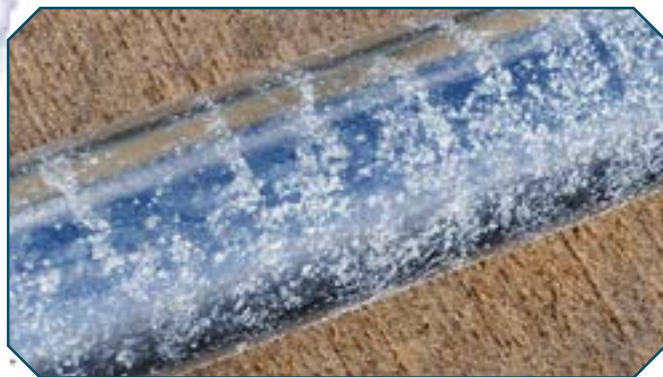
Figure 8: Medium wet storage stain
