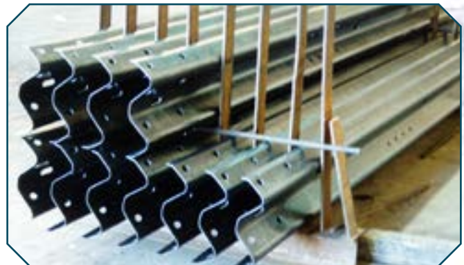
Figure 6: Storage of galvanized steel, utilizing spacers to increase freely flowing air
