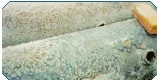
Figure 9: Heavy wet storage stain
