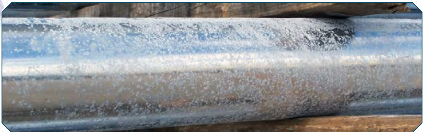
Figure 3: Extremely high moisture condition
