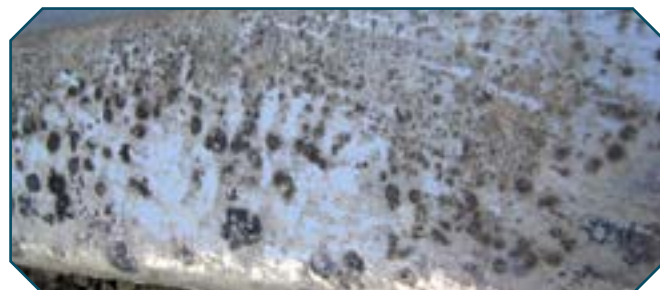
Figure 10: Extreme wet storage stain
