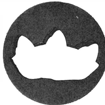
(D) contacting surface of spline teeth wear away by fretting corrosion
