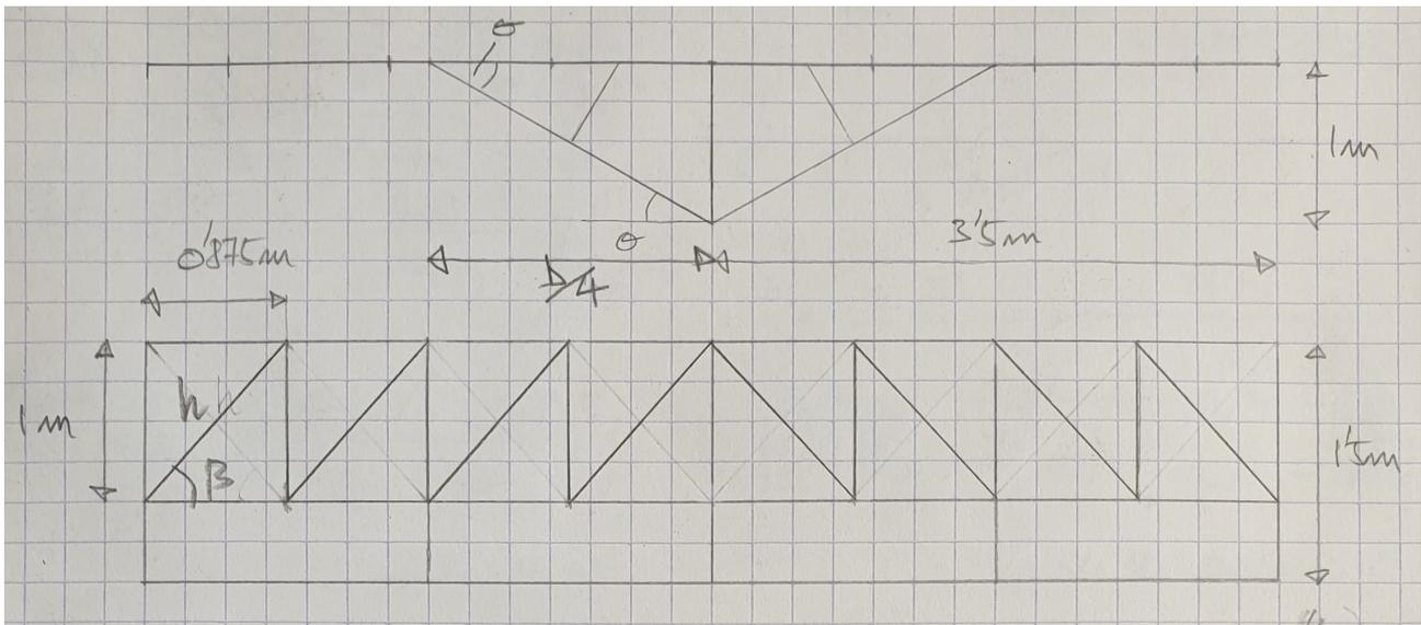
Front and top view of the tube and fabric basic glider wing structure.
