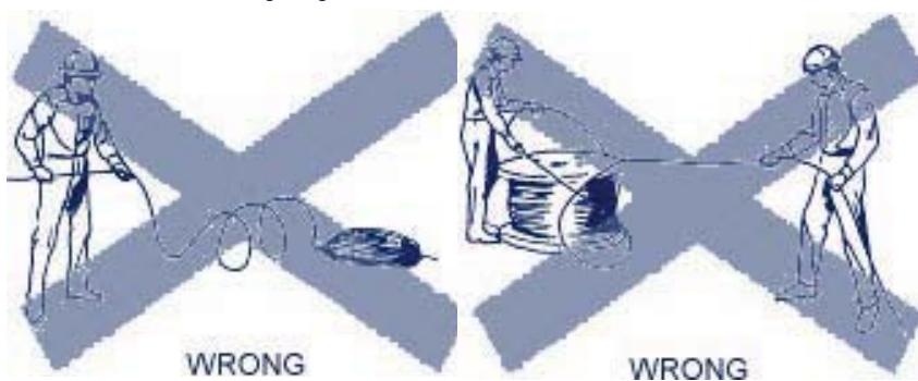
Figure 7. Illustrations of a wrong method of unreeling wire rope.
