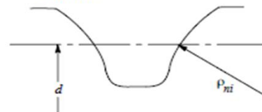
Figure A-1 - Radius of normal thread profile ZI
