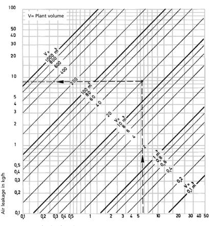
Vacuum loss in mbar/min (The diagram is valid for pressures  $\leq$  500 mbar and for air of 20 °C)
