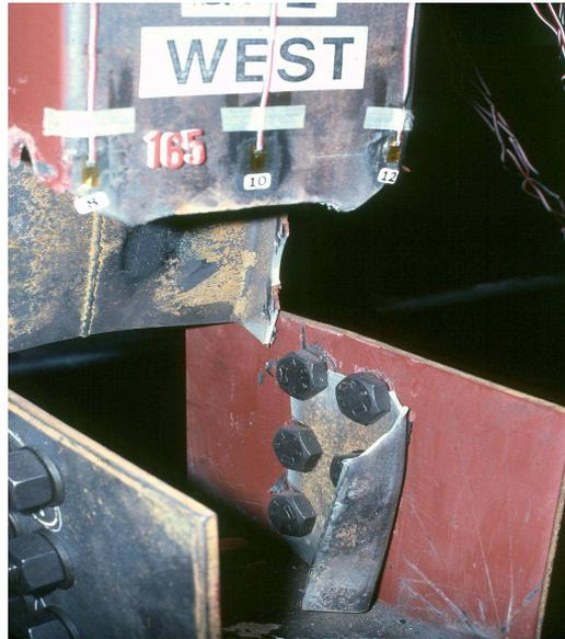
Figure 8.11 – Tear out failure mode for a bolted RHS (with a hand access hole cut-out) in tension
