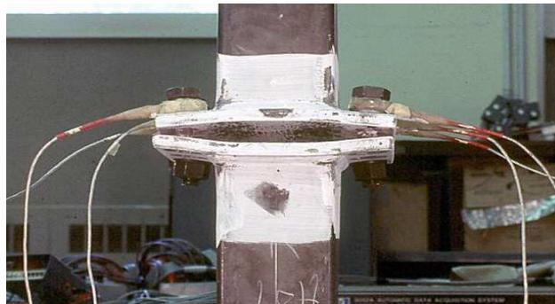
Figure 8.4 – Tension test of a flange-plate joint bolted along two RHS sides, showing plate flexure
