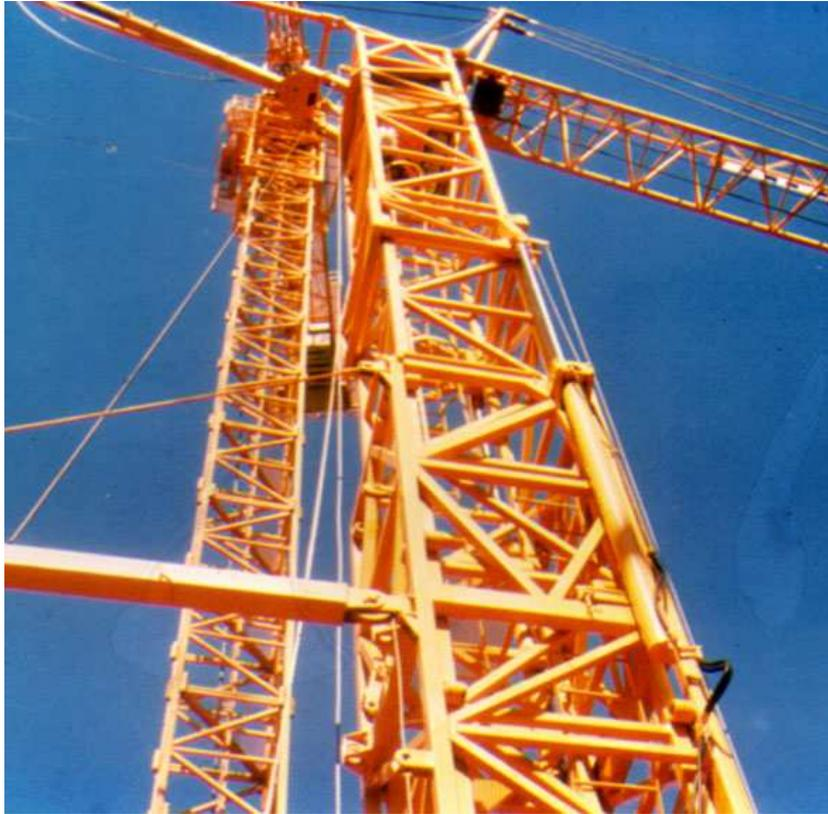
Figure 2.4 – Rectangular hollow sections used in a crane
