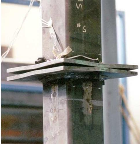
Figure 8.7 – Tension test of a flange-plate joint bolted along one side of an RHS (four bolts; thin plates)
