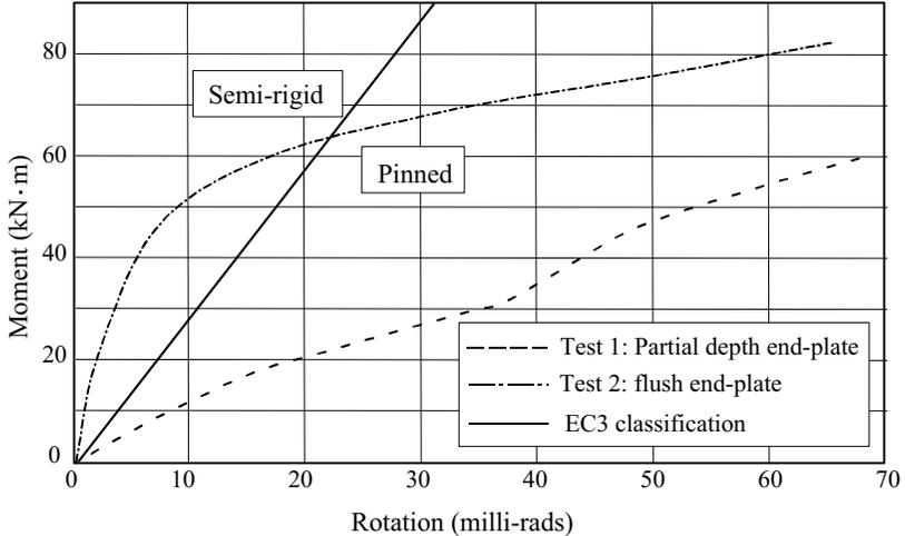
Figure 6.37 – Moment rotation curves of a flush and a partial depth endplate connection
