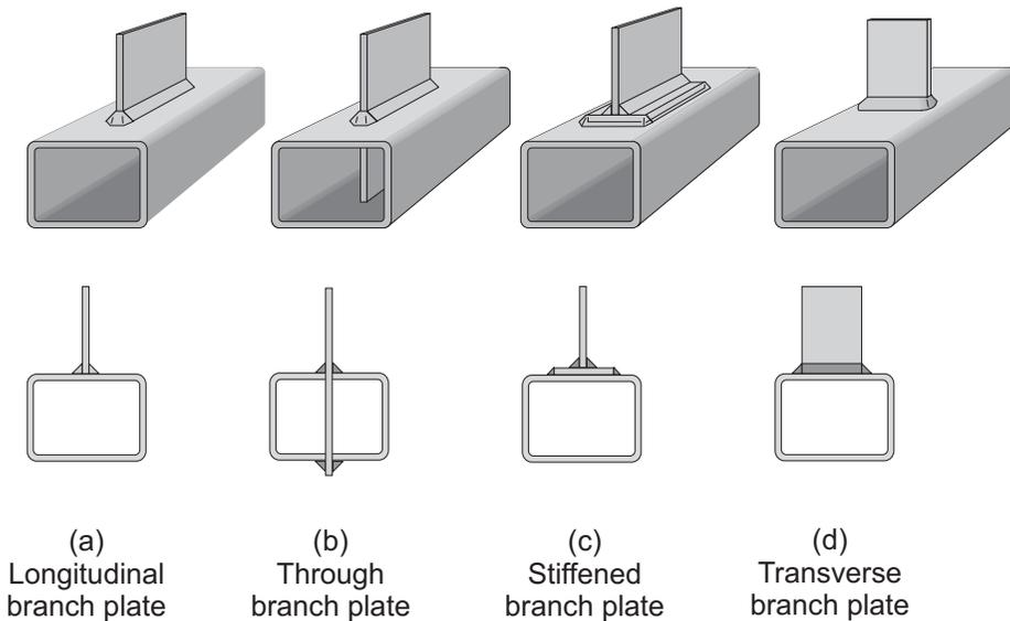
Figure 10.4 – Branch plate-to-RHS member connection types
