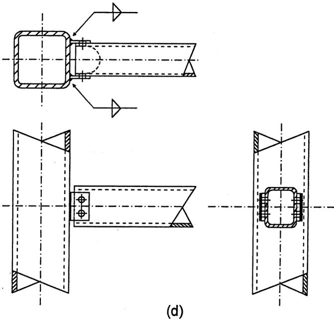
Figure 5.12 – Simple shear connections with hollow section beams
