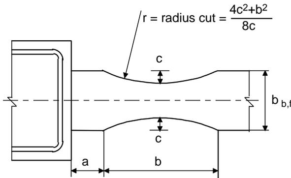
Figure 8.14 – Geometry of radius cut RBS
