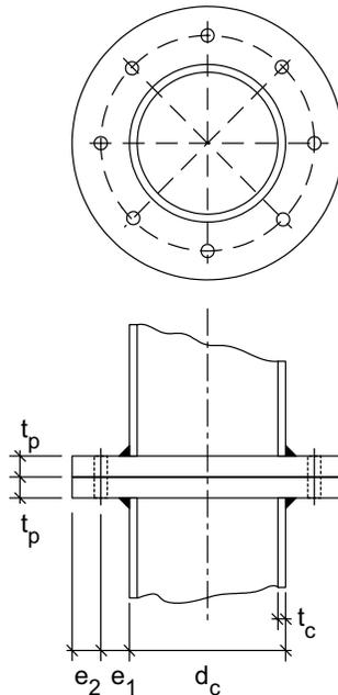
Figure 11.1 – Circular column with site bolted end plates
