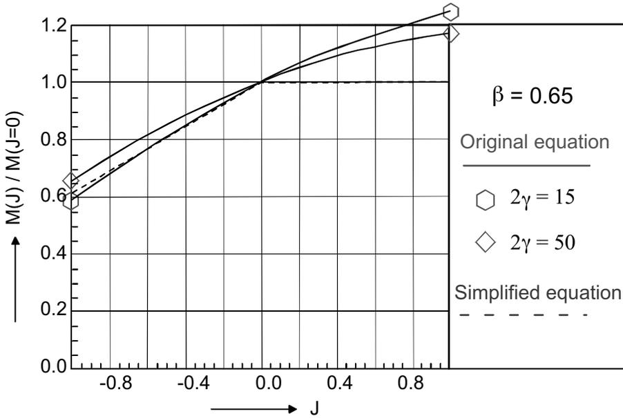
Figure 6.16 – Multiplanar effect of I-beam-to-CHS column connections loaded by in-plane-bending moments ( $\beta = 0.65$ )
