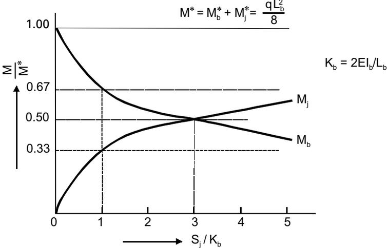
Figure 4.2 – Variation of elastic moment distribution with connection stiffness (Anderson et al. 1997)
