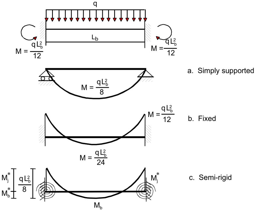
Figure 4.1 – Beam with various end conditions
