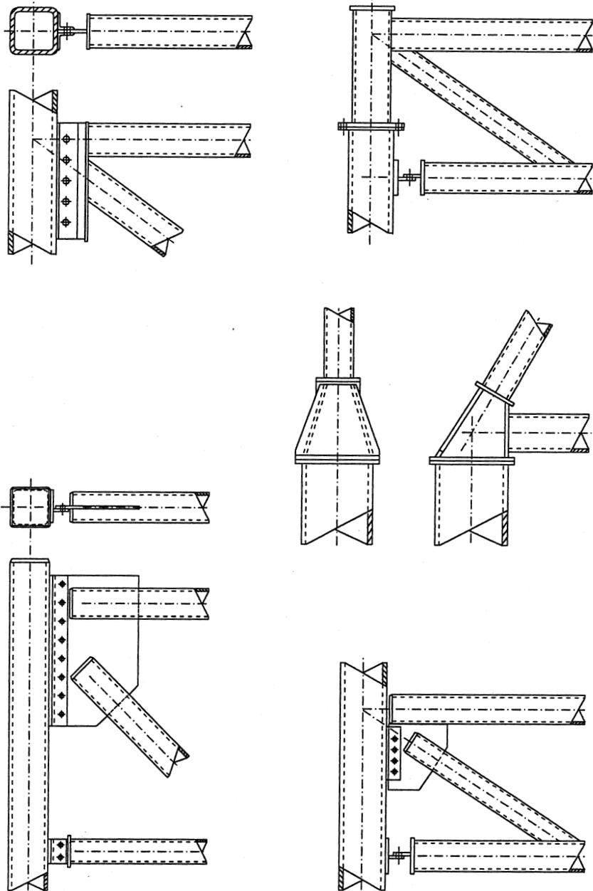
Figure 10.8 – Typical truss to hollow section column connection arrangements
