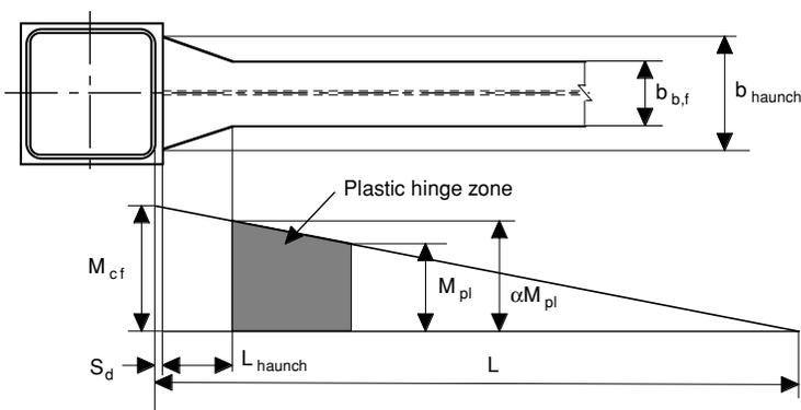
Figure 8.10 – Beam-to-column connection with horizontal haunches
