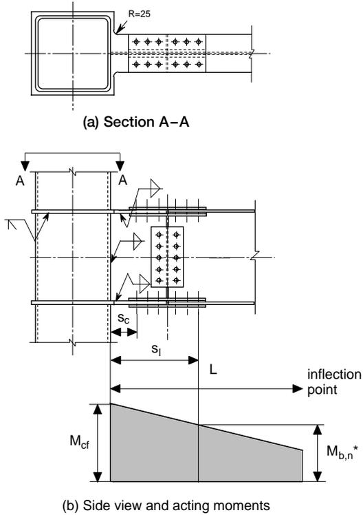
Figure 8.5 – Bolted through diaphragm connections
