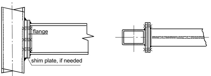
Figure 6.23 – Bolted flange plate connection between RHS members
