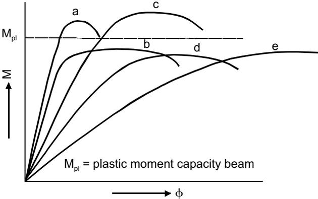
Figure 4.3 – Various M-φ characteristics
