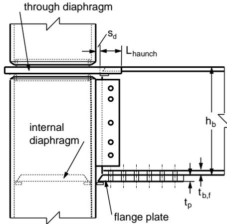
Figure 8.19 – Beam-to-column connections with combined internal and through diaphragms
