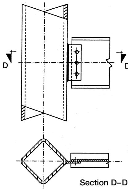
Figure 5.5 – Single shear plate connection to corner of rectangular column
