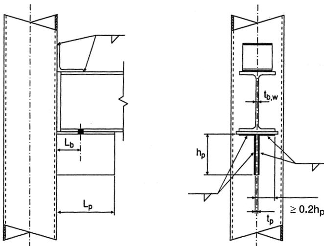
Figure 5.11 – Stiffened seat connection
