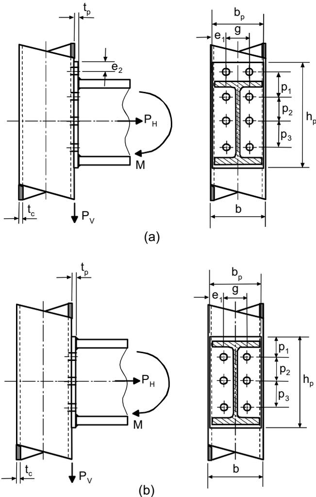
Figure 6.27 - Blind bolted I-beam-to RHS column connections
