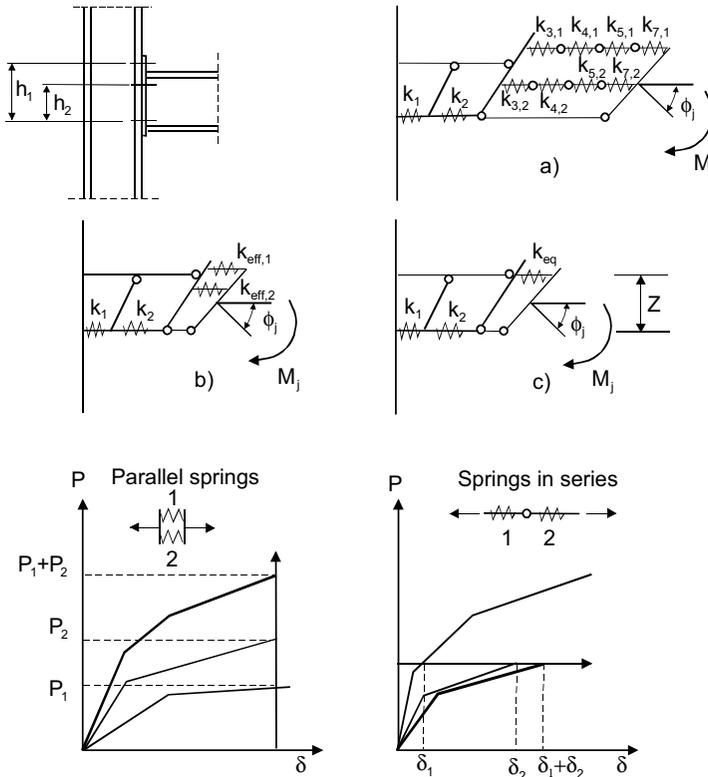
Figure 4.10 – Examples of spring models used for a bolted beam-to-column connection with an end plate (Jaspart 1997)
