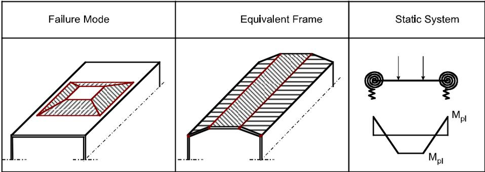
Figure 4.9 – Simplified frame for component behaviour
