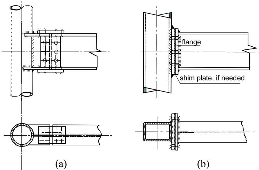
Figure 6.26 - Bolted beam-to-column connection with a continuous column
