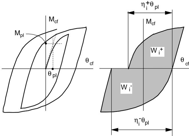
Figure A.7 – Definition of cumulative plastic deformation factor
