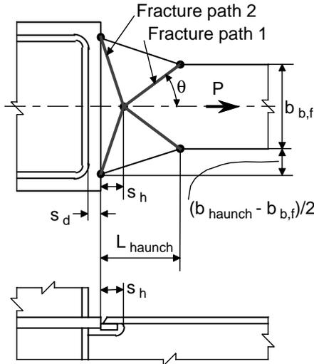
Figure 8.11 – Fracture paths in horizontal haunches
