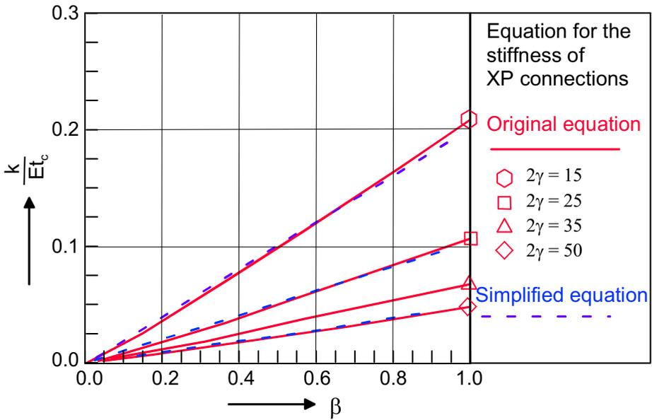
Figure 6.12 – Stiffness of XP-1 connections
