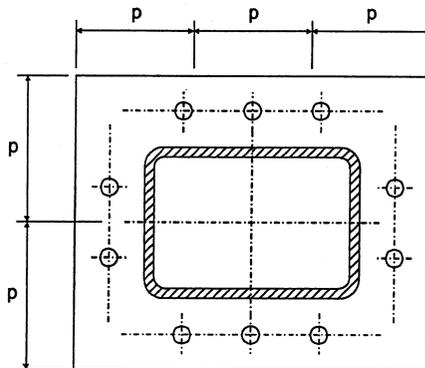
Figure 11.3 – Definition of bolt pitch  $p$  for RHS flange-plate connections
