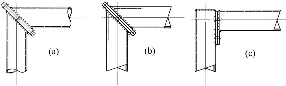
Figure 6.22 – Bolted knee assemblies of CHS or RHS members for portal frames
