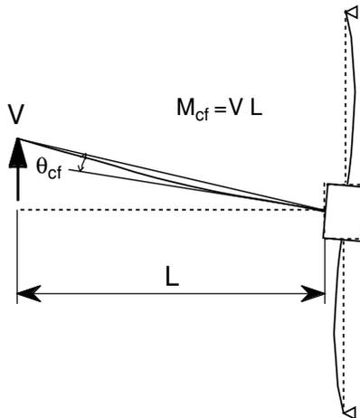
Figure A.6 – Definition of beam rotation and moment at column face
