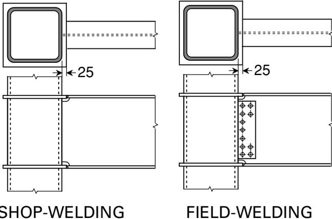
Fig A.1 – Examples of conventional connection designs
