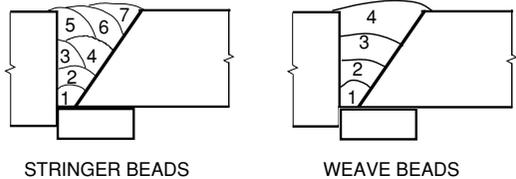
Figure A.3 – Cross section of weld beads
