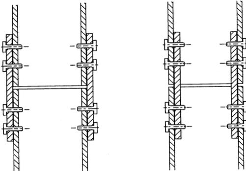
Figure 11.4 – Bolted side plates (left external, right internal)
