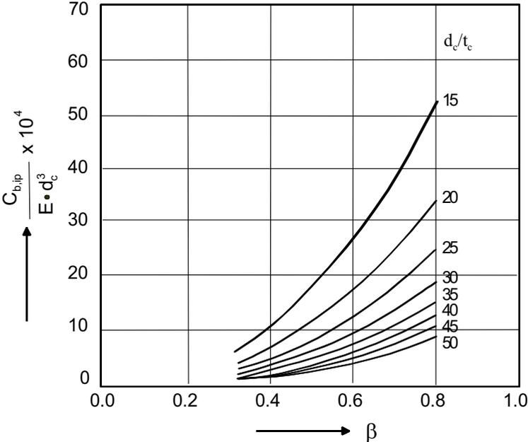
Figure 6.31 - Connection stiffness for T-connections between CHS members
