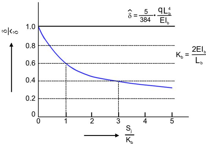
Figure 4.4 – Variation of mid-span deflection with connection stiffness (Anderson et al. 1997)
