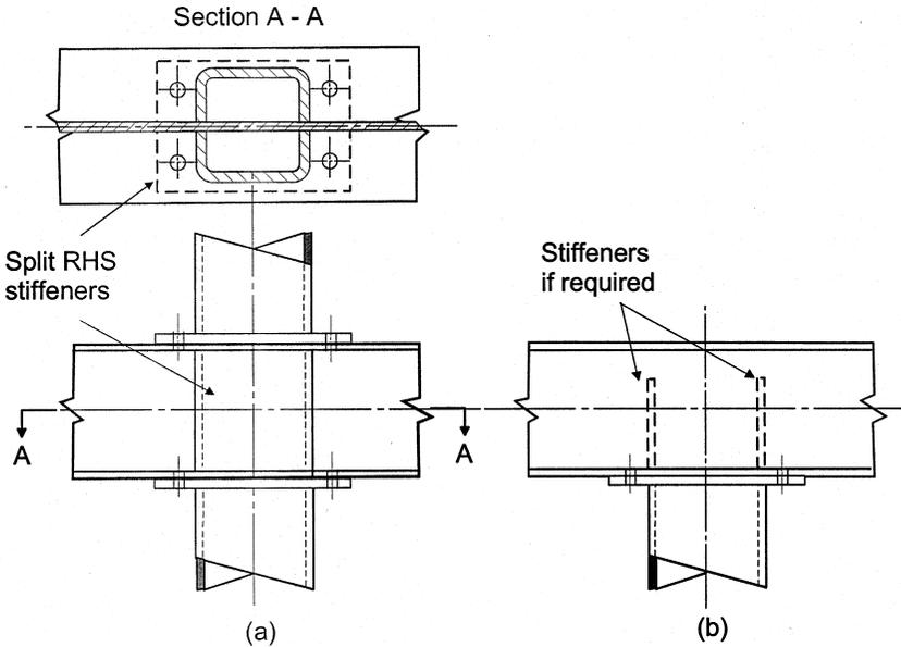
Figure 6.24 – Bolted continuous beam-to-column connections (Packer and Henderson, 1997)
