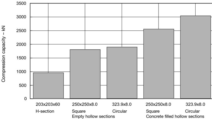
Figure 2.4 – Compression capacities for sections of equal mass (about 60 kg/m) with concrete filling
