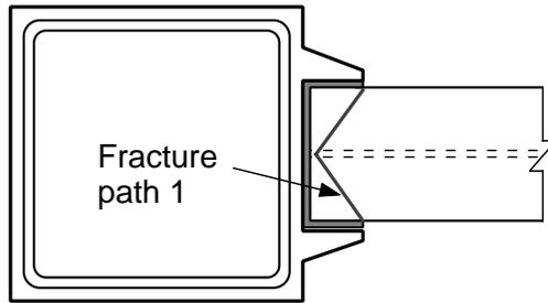
Figure 8.13 – Connection with U-shaped welded joints
