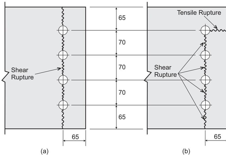
Figure 5.2 – Two possible failure paths for net section fracture in shear plate
