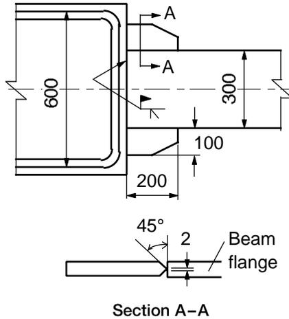
Figure 8.12 – Details of welded horizontal haunches
