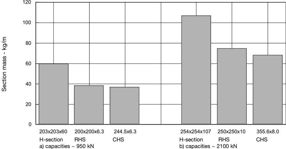
Figure 2.3 – Comparison of section masses for equal compression capacities
