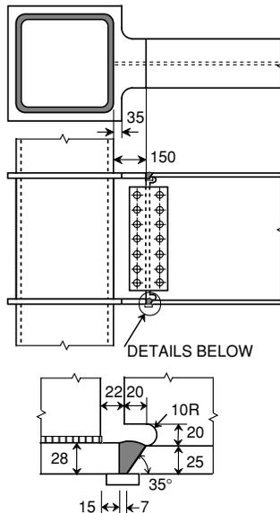
Figure A.2 – Improved connection for field-welding applications
