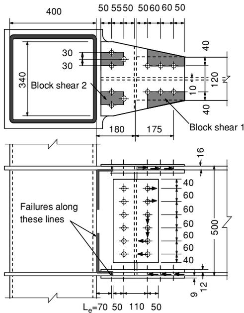
Figure 8.6 – Design example and assumed failure modes of beam splice and stub-beam
