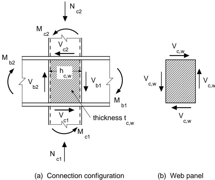
Figure 7.5 – Column web panel framed by flanges and stiffeners
