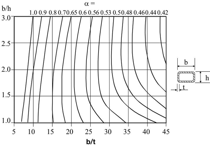
Figure 6.9 – Stress reduction factor  $\alpha$ , for  $90^\circ$  unstiffened mitred RHS knee connections subjected to bending about the minor axis
