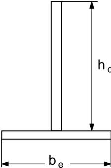
Figure 9.6 – Critical steel section through diaphragm and column wall
