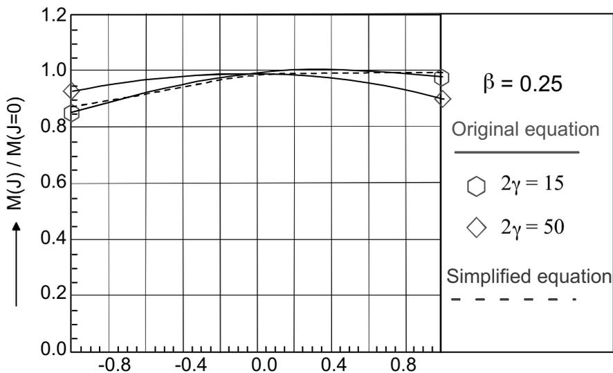
Figure 6.14 – Multiplanar effect of I-beam-to-CHS column connections loaded by in-plane-bending moments ( $\beta = 0.25$ )
