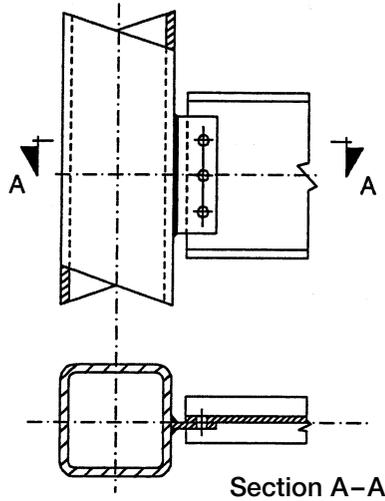
Figure 5.1 – Single shear plate connection
