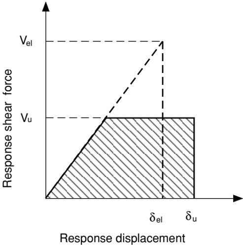
Figure 7.1 – Load displacement relationships of elastic and inelastic structure under impulsive loading
