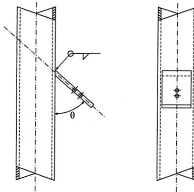
Figure 10.7 – Inclined transverse branch plate welded to the “flat” of a RHS column
