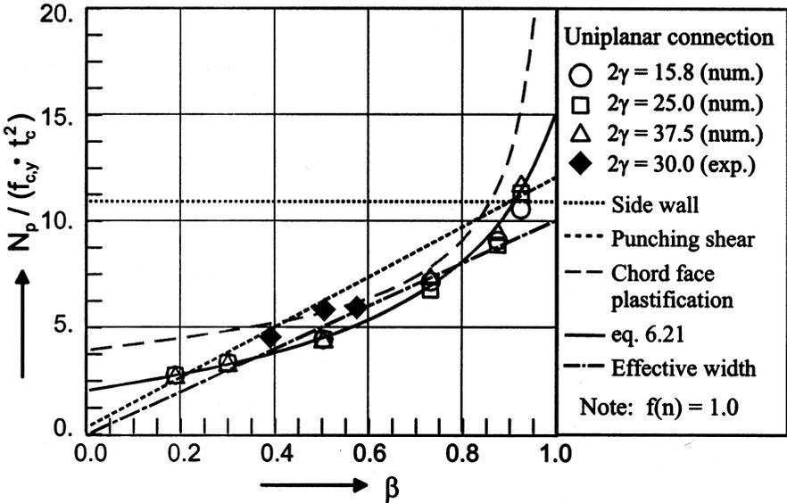
Figure 6.18 – Comparison of the FE results based on the 3% of the column width  $b_c$  deformation criterion and the column face yield line criterion, the punching shear criterion, the plate effective width and column side wall criterion (Lu, 1997)
