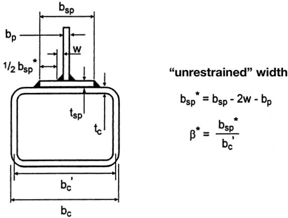
Figure 10.6 – Nomenclature for stiffened longitudinal branch plate connections to RHS
