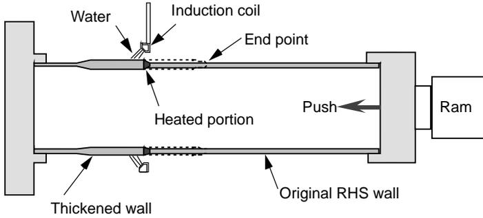
Figure 8.23 – Manufacturing process for partially thickening sections
