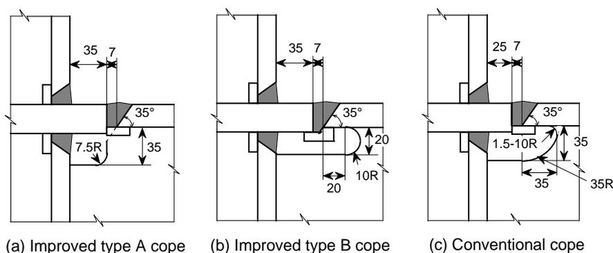
Figure 8.2 – Details of improved and conventional beam copes
