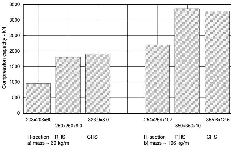
Figure 2.2 – Comparison of compression capacity for sections of equal mass
