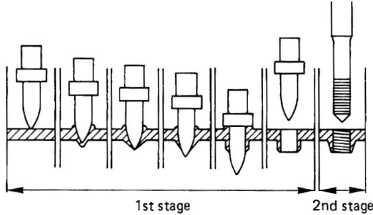
Figure 3.1 – Schematic of the Flowdrill process
