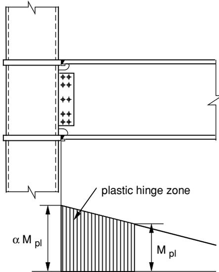
Figure 7.4 – Example of beam-to-column assemblies with conventional details
