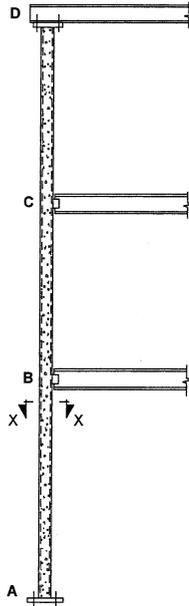
Figure 9.1 – Recommended method for introducing beam shear reactions to concrete filled columns at roof and floor levels.
