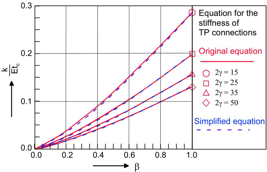
Figure 6.13 – Stiffness of TP-1 connections
