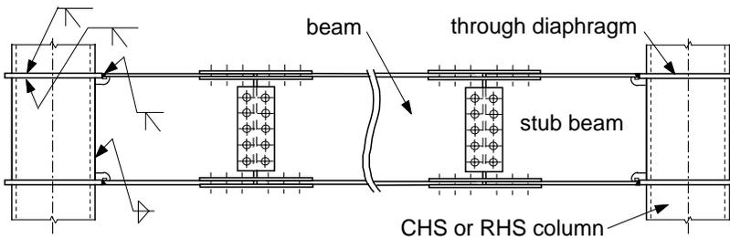
Figure 8.1 – Beam-to-column connections with through diaphragms for shop-welding
