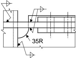
(c) Details of welded joints at flange centre
