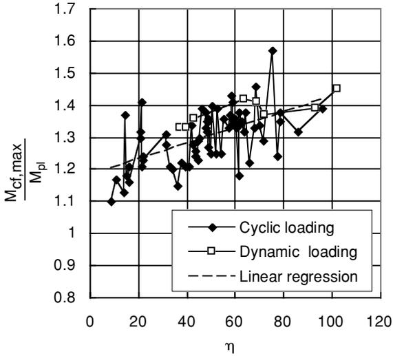
Figure A.5 – Overstrength factor compared with cumulative plastic deformation factor (AIJ Kinki 1997)
