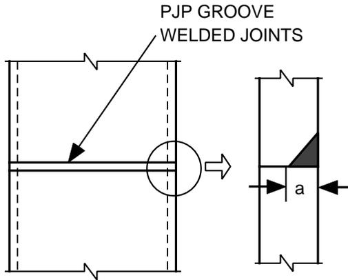
Figure 11.6 – Column splice with PJP welded joint
