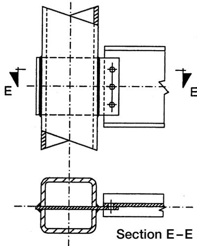
Figure 5.6 – Through-plate connection
