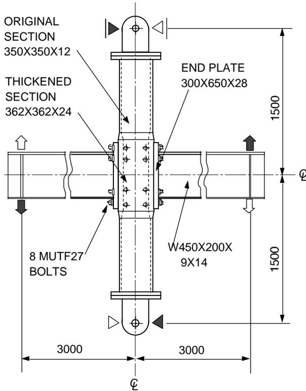
Figure 8.24 – Schematic diagram for anti-symmetric loading
