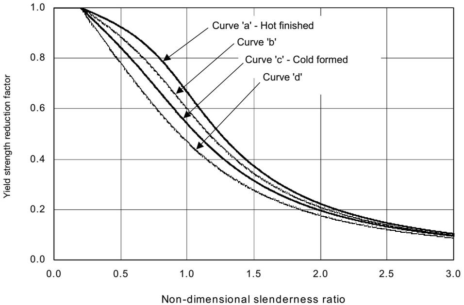
Figure 2.1 – Eurocode 3 column buckling curves
