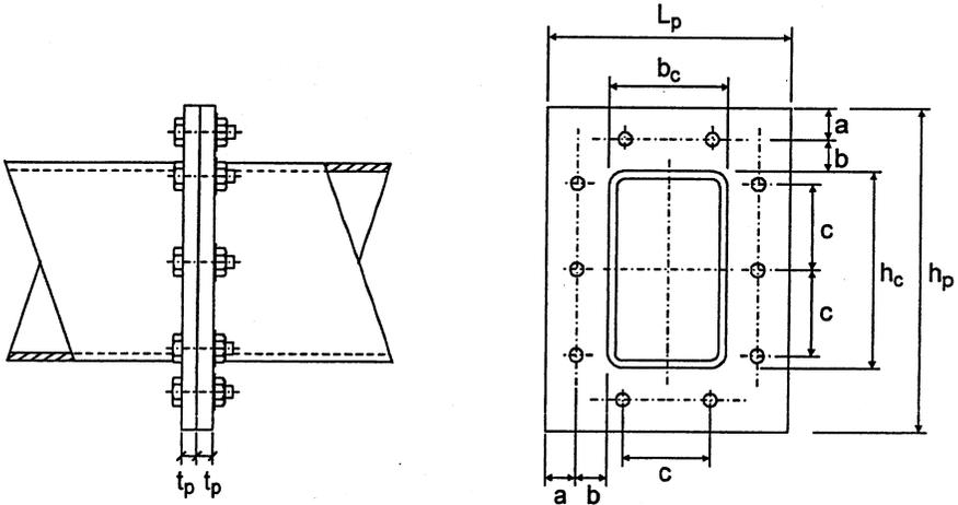
Figure 11.2 – Layout of site-bolted RHS column flange-plate connection
