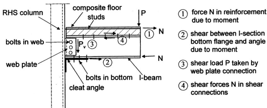
Figure – 9.4 Resisting forces in the connections of figures 9.2 and 9.3
