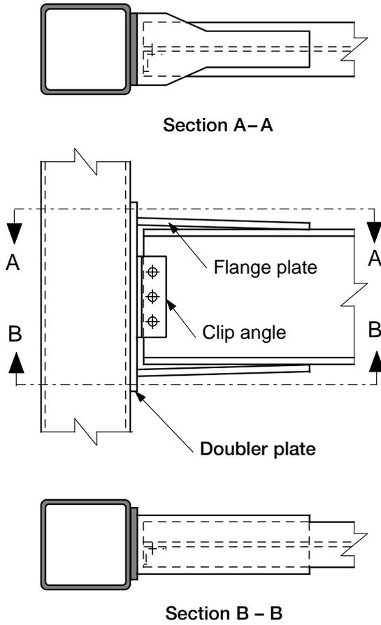
Figure 8.25 – Beam to column connection with doubler plates
