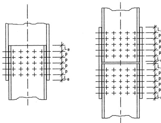
Figure 11.8 – Splice connection using shot fired nails
