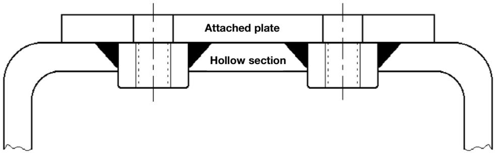
Figure 3.4 – Nuts welded into hollow section wall
