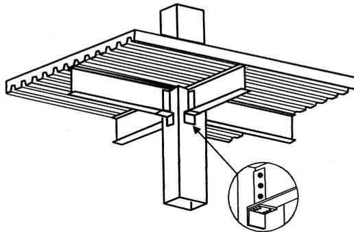
Figure 9.3 – Connection of an I-beam with a concrete slab to a (concrete filled) RHS column
