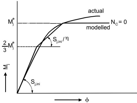
Figure 4.6 – M- $\phi$  modelling according to Eurocode 3: Annex J
