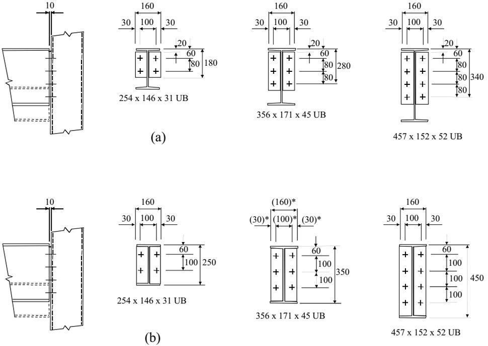
Figure 6.36 – I-beam-to-RHS column connection with partial depth and flush endplates (France et al.1999, 1999a)
