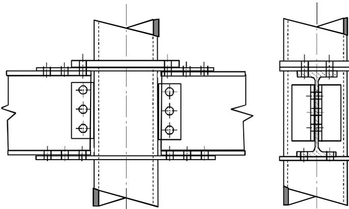
Figure 6.25 – Bolted through-plate moment connections (Packer and Henderson, 1997)
