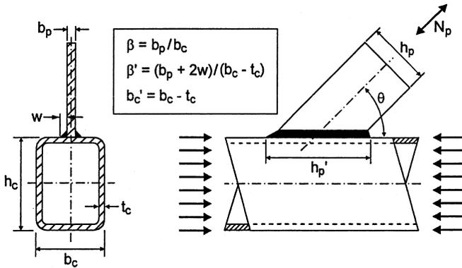
Figure 10.2 – General longitudinal plate-to-RHS member connection
