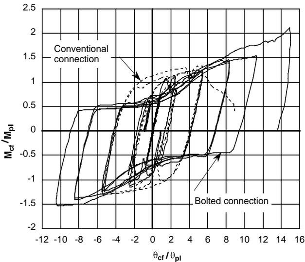
Figure 8.7 – Comparison of moment/rotation hysteretic curves between conventional and bolted through diaphragm connections
