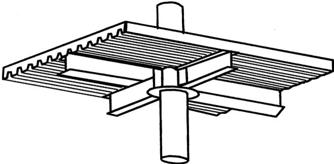
Figure 9.2 – Connection of an I-beam with a concrete slab to a (concrete filled) CHS column
