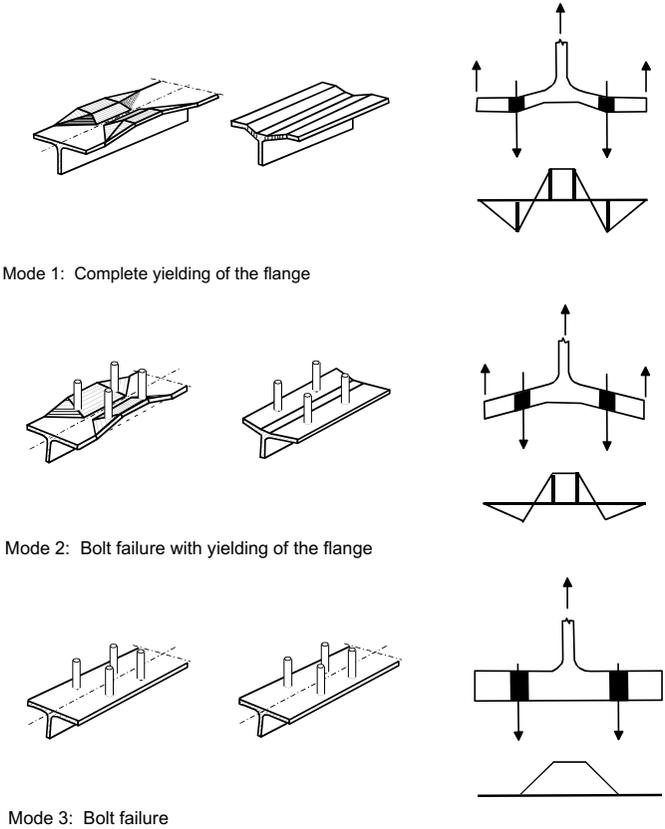
Figure 4.8 – Failure modes of actual components and equivalent T-stub flanges for bolted beam-to-column connections (I-beams)
