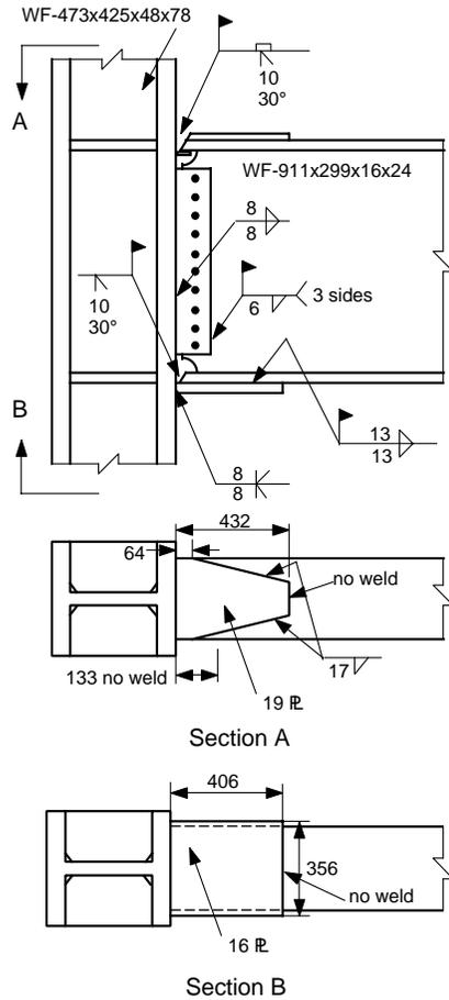
Figure 8.18 – Beam-to-column connection with cover plates (Engelhardt and Sabol 1998)
