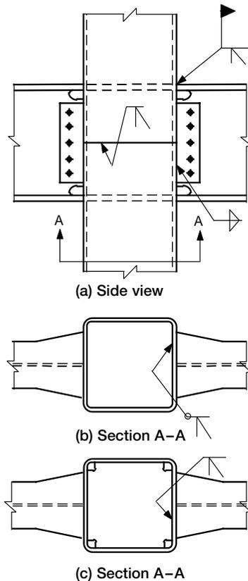
Figure 8.15 – Beam-to-column connections with internal diaphragms
