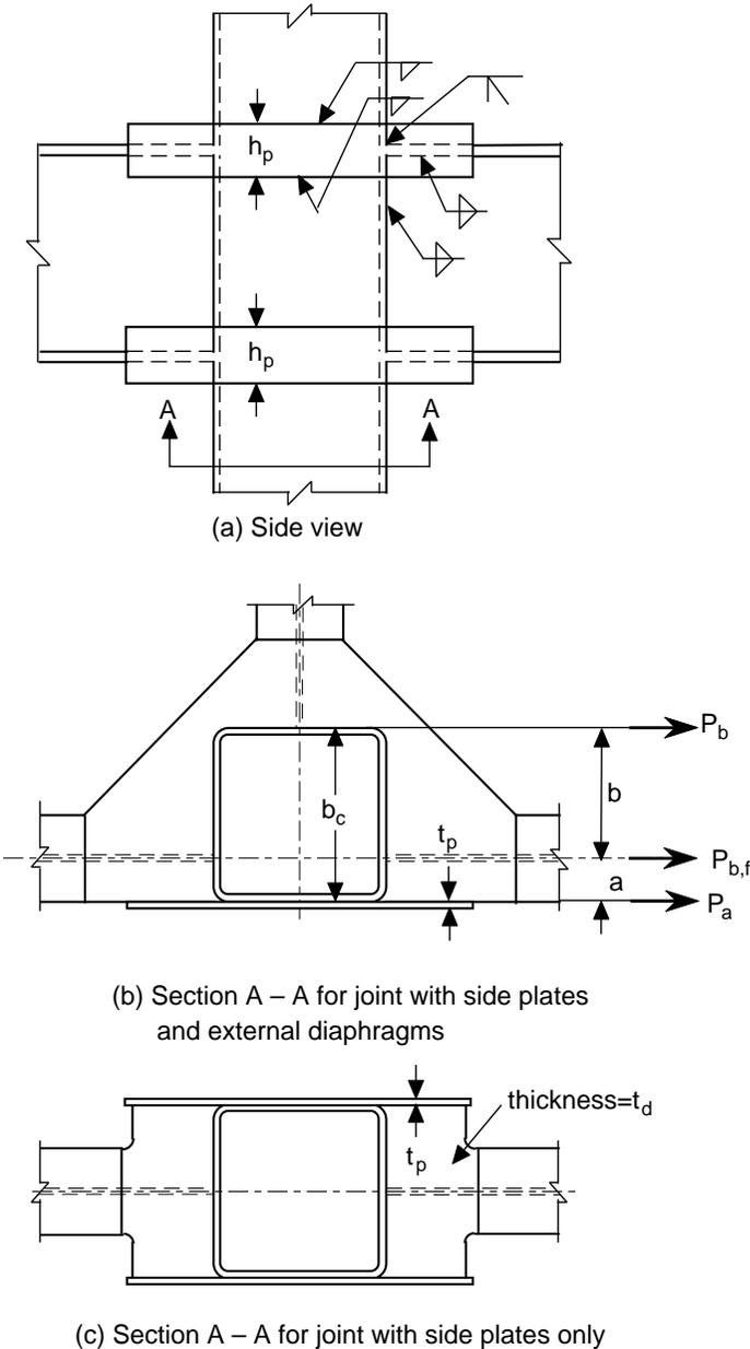
Figure 8.21 – Beam-to-column connections with external diaphragms and side plates
