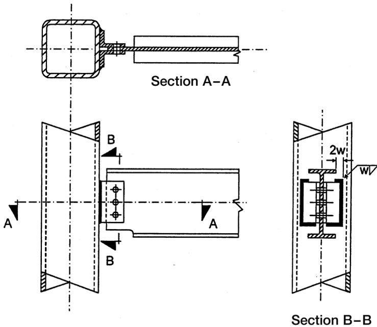
Figure 5.9 – Double angle connection
