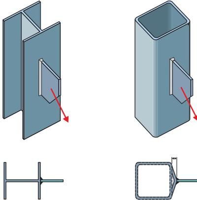
Figure 10.1 – Longitudinal branch plate connections in braced structures
