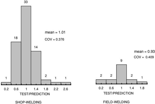
Figure A.4 – Histograms showing distributions of test to predicted ratios
