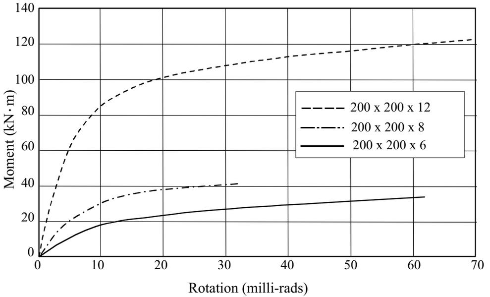
Figure 6.38 – Moment-rotation curves of flush endplate connections between a 356 UB and RHS columns with varying thickness
