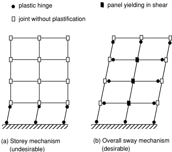
Figure 7.3 – Comparison of desirable and undesirable collapse mechanisms
