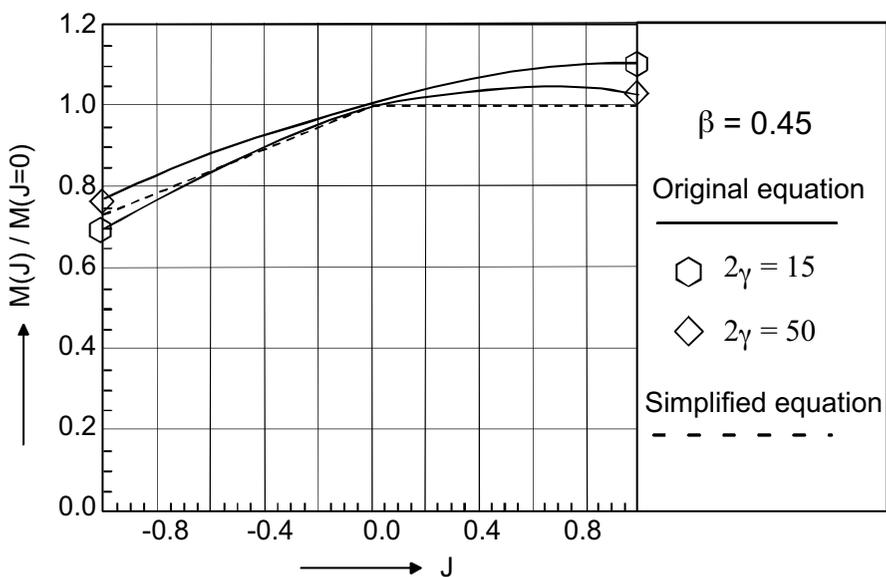
Figure 6.15 – Multiplanar effect of I-beam-to-CHS column connections loaded by in-plane-bending moments ( $\beta = 0.45$ )
