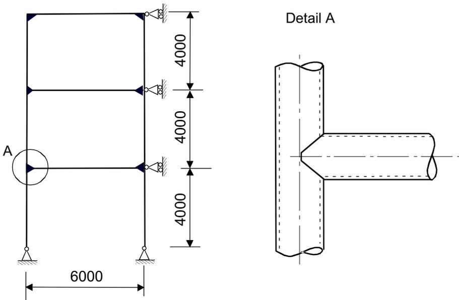
Figure 6.30 – Frame of CHS beams and columns
