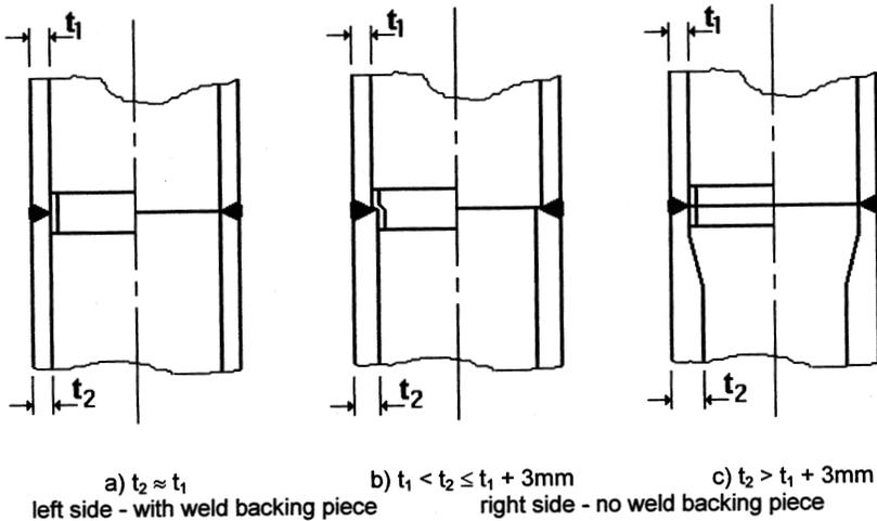
Figure 11.5 – Plane column splices – site welding with a weld backing piece
