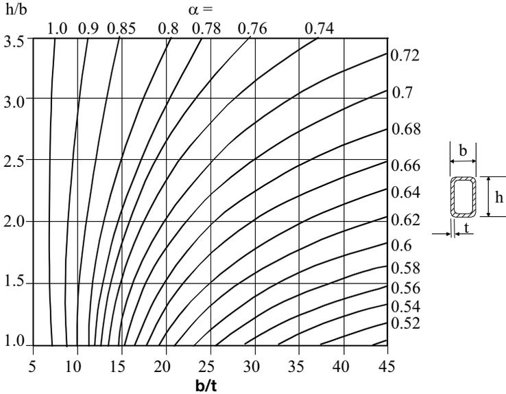
Figure 6.8 – Stress reduction factor  $\alpha$ , for  $90^\circ$  unstiffened mitred RHS knee connections subjected to bending about the major axis
