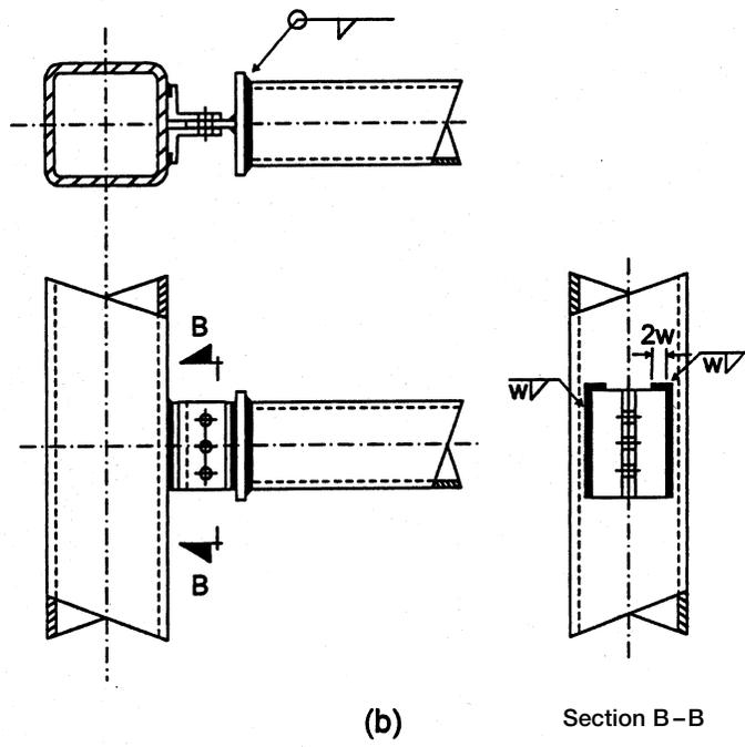
Figure 5.12 – Simple shear connections with hollow section beams
