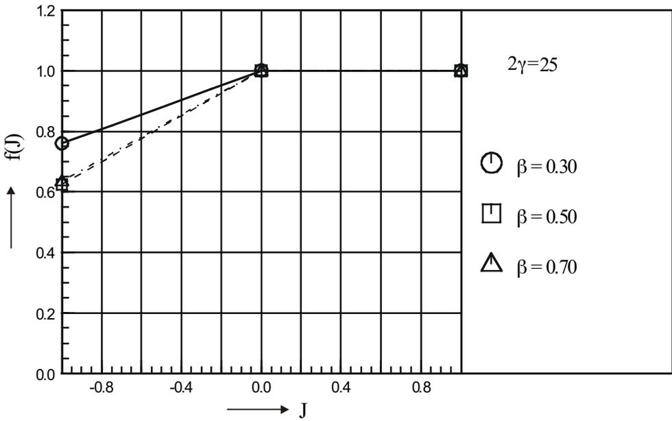
Figure 6.20 – Multiplanar loading effect for I-beam-to-RHS column moment connections
