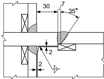
Figure 8.4 – Further improvement in beam end cutting with no access hole
