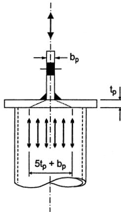
Figure 10.3 – Load dispersion for T-stub connection on the end of a CHS member
