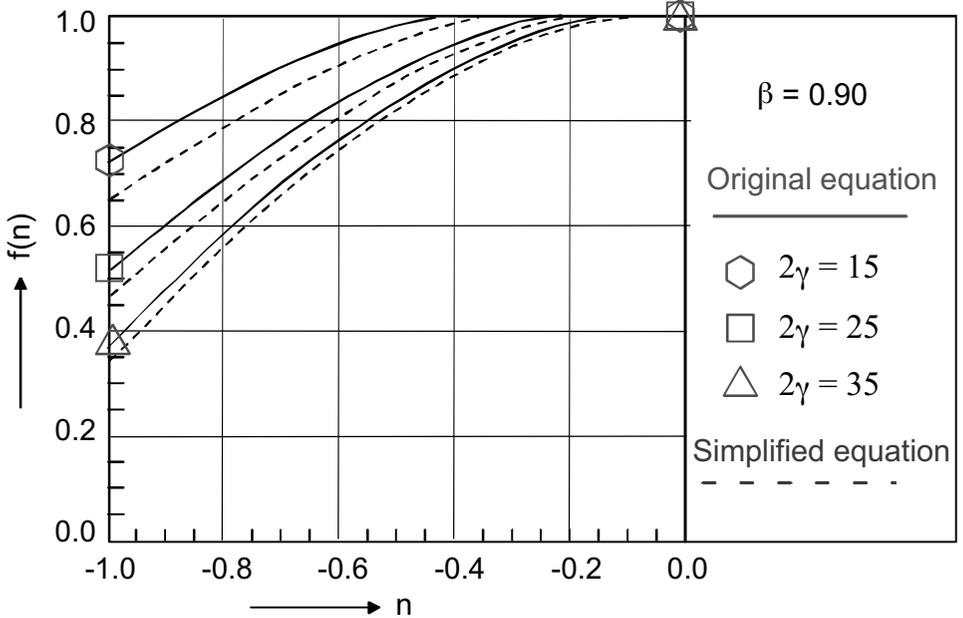
Figure 6.19 – Effect of column loading on the connection moment resistance
