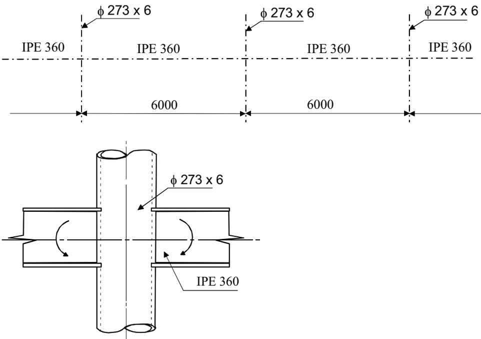
Figure 6.35 – Welded connection between the IPE 360 and the CHS 273 x 6
