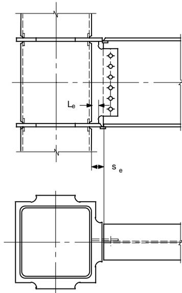
Figure 8.9 – Improved field-welded connection
