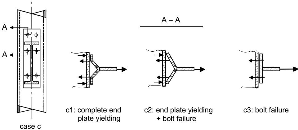
Figure 6.29 - Plate plastification models
