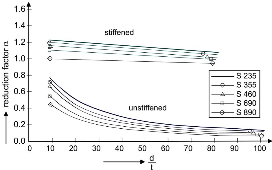
Figure 6.4 – Stress reduction factor  $\alpha$ , for unstiffened mitred CHS knee connections
