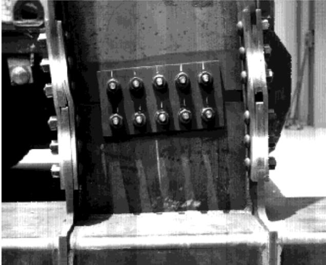
Figure 8.8 – Failure mode of bolted through diaphragm connection
