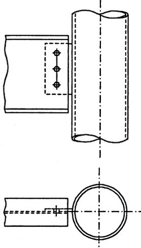
Figure 5.3 – Single shear plate connection to CHS column
