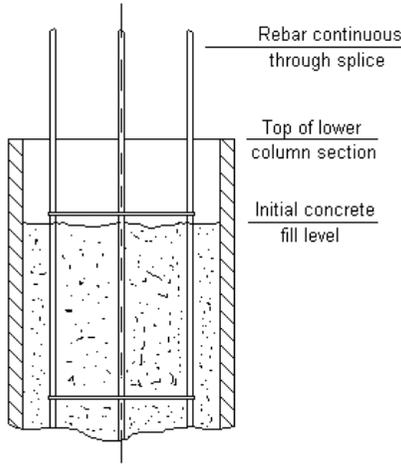
Figure 11.7 – Concrete filled column splice, with continuity of concrete and rebar
