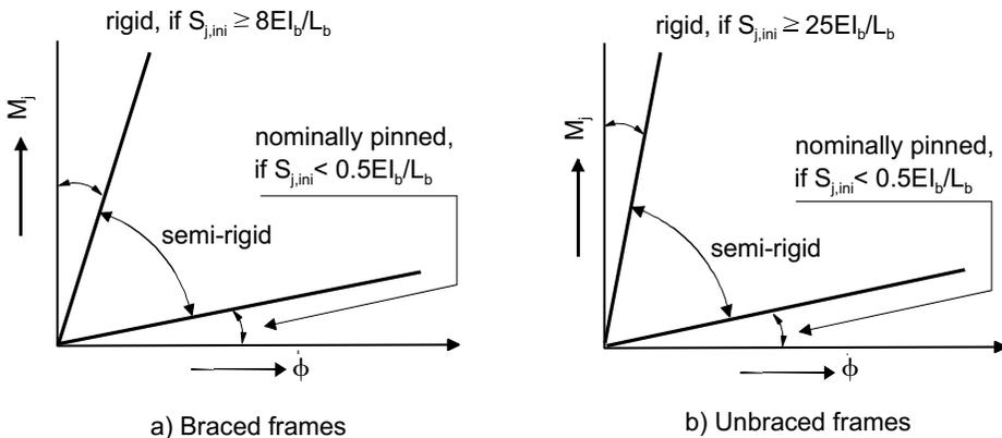
Figure 4.7 – Boundaries for stiffness classification of beam-to-column connections (EC3, Annex J)
