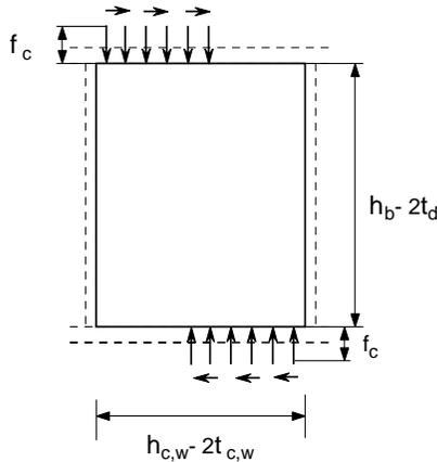
Figure 9.5 – Stresses in concrete panel
