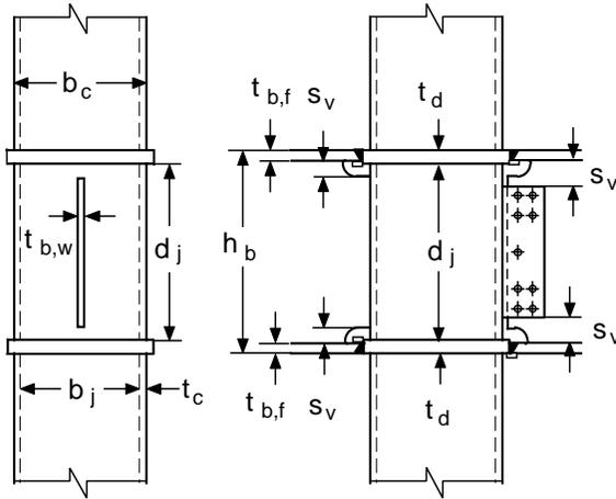
Figure 8.3 – Dimensions of welded web joint
