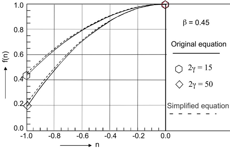
Figure 6.17 – Influence of column stress on I-beam-to-CHS column connections loaded by in-plane-bending moments ( $\beta = 0.45$ )
