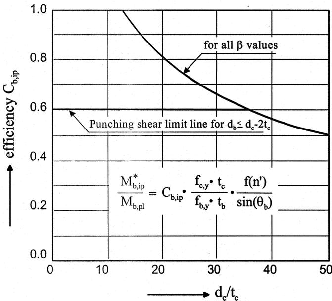
Figure 6.32 – Design graph for CHS connections loaded by in-plane bending moments
