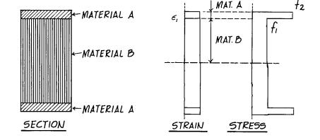
In flexure, if the two materials are at the same distance from the N.A., they will have the same strain at that point. Therefore, the strains are "compatible".
