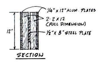
WOOD:  $E = 1.5 \times 10^3$  K.S.I. STEEL:  $E = 30 \times 10^3$  K.S.I. ALUM:  $E = 12 \times 10^3$  K.S.I
