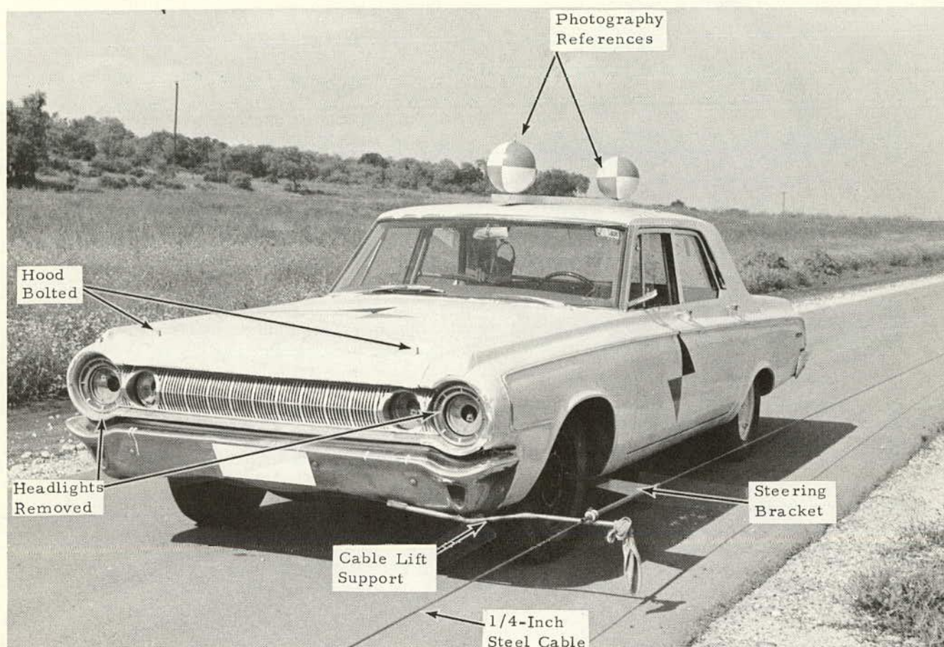
Figure A-2. Guide bracket on typical test vehicle.
