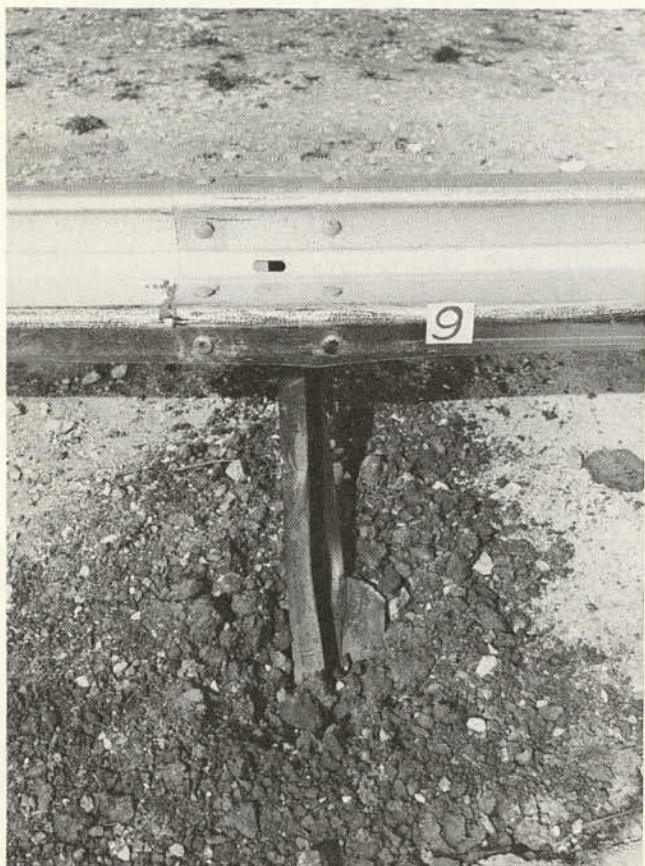
Figure A-16. Guardrail Posts 7, 8, and 9, and terminal end, after Test 105.
