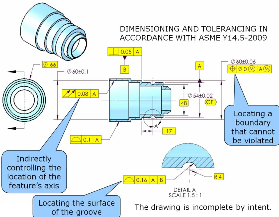
The drawing drives the entire process. When the drawing is unclear it affects purchasing, tooling, quality plans, assembly, inspection software, tolerance analysis software, etc. The Y14.5 standard has been proven to have only one meaning. To continue to ignore this Standard is irresponsible.
