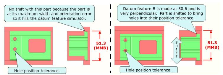
Datum feature B of the part on the left was produced at its largest size and with maximum allowable perpendicularity error. It just fills the datum feature simulator and would not be able to shift around in a fixture. The holes illustrated are out of position tolerance.
