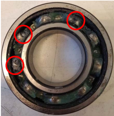
Fig. 2. Detail of damage 1 (three cage/ball positions drilled)
