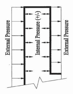
External and Internal Parapet Pressures
