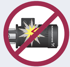
Fig 1.4.5: For increased safety motors EExe, no sparks may occur. The temperature classification covers both internal and external surfaces.
