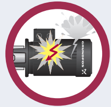
Fig 1.4.4: The explosion occurs inside the motor and is lead out of the motor through the flame paths. The temperature classification for flameproof EExd motors is valid for external surfaces.
