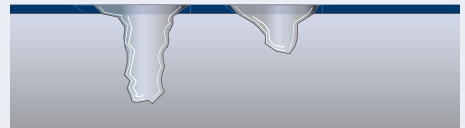
Fig. 1.6.4: Pitting corrosion
