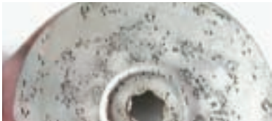
Pitting corrosion of EN 1.4401 (AISI 316)
