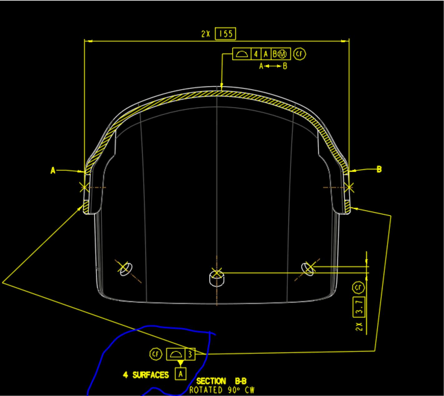
2. 4X Datum B is applied but in 4 holes which hole axis is oriented with particular datum A face is not clear
